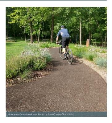
and cost. For these reasons, rubberized trail tread has rarely been used on mountain bike trail systems. On the plus side, rubberized tread has excellent traction characteristics, drains extremely well, and is available in multiple color options. Rubberized trail tread is commonly used in playgrounds and sidewalk-style applications.
