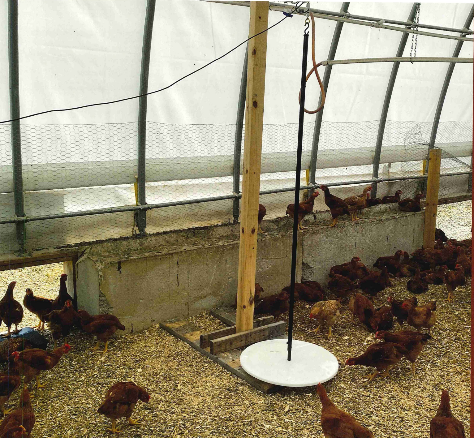
Poultry live scale system installed in a coop.
