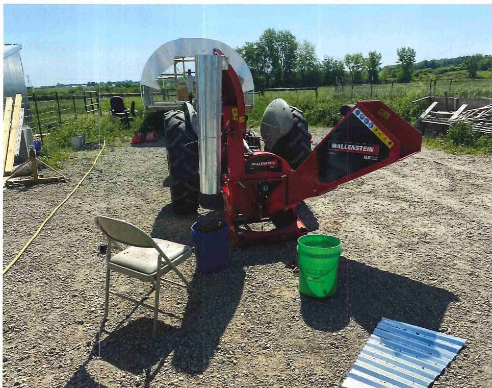
PTO driven woodchipper used to process hazelnuts.
