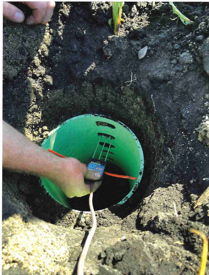
Soil moisture sensor installed in the field.
