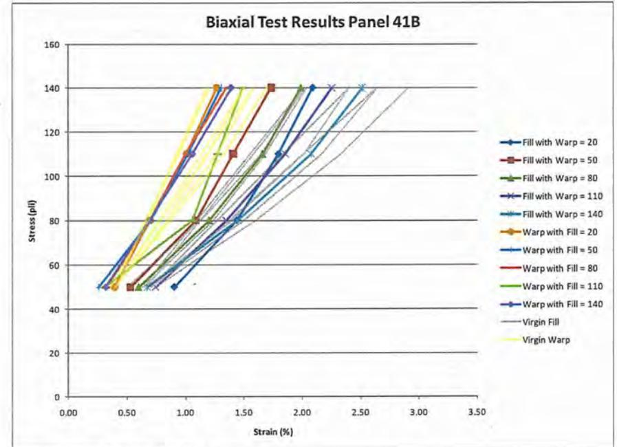
Figure 13: Panel 41B Biaxial Test Results
