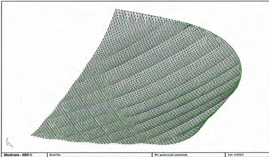
Figure 2: Roof Model Deflated Position
