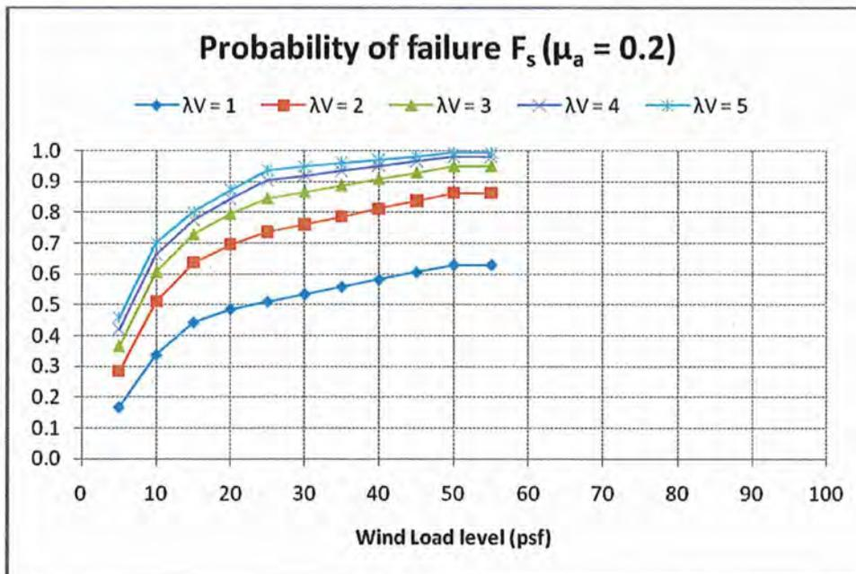
Figure 8 Probability of rectangular panel failure under wind load, mean flaw size 12 mm
