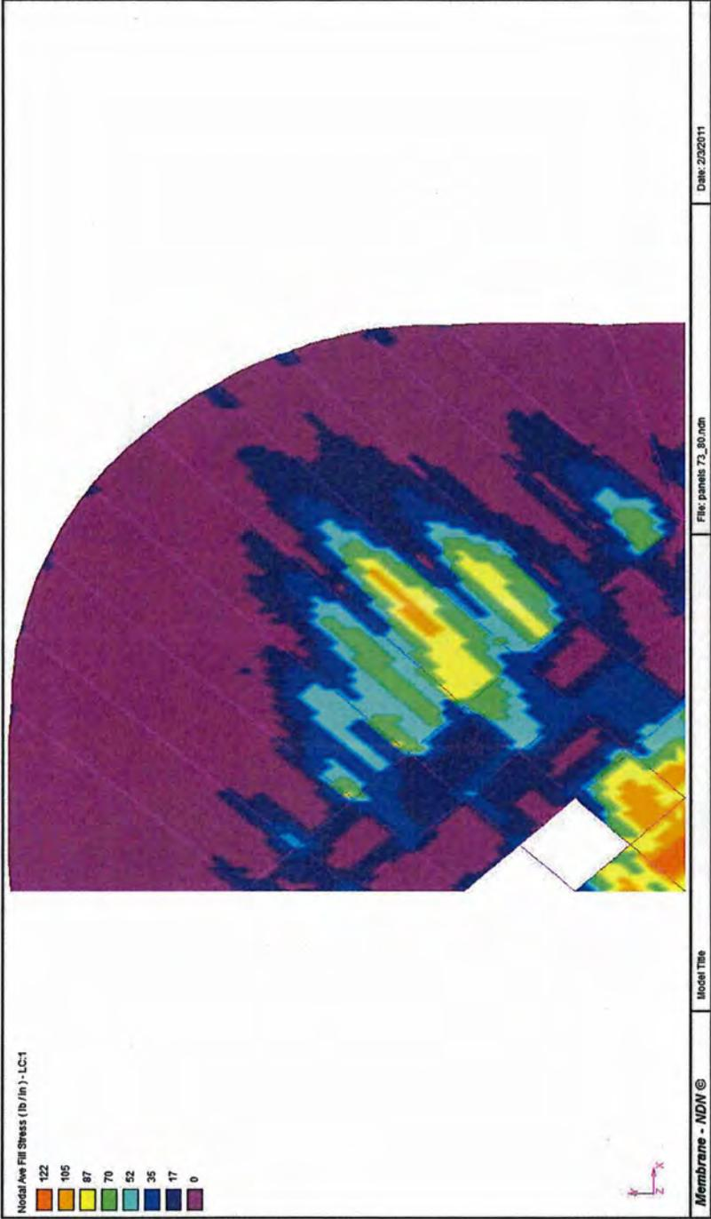
Figure 13 Panels 73-80 fill stresses
