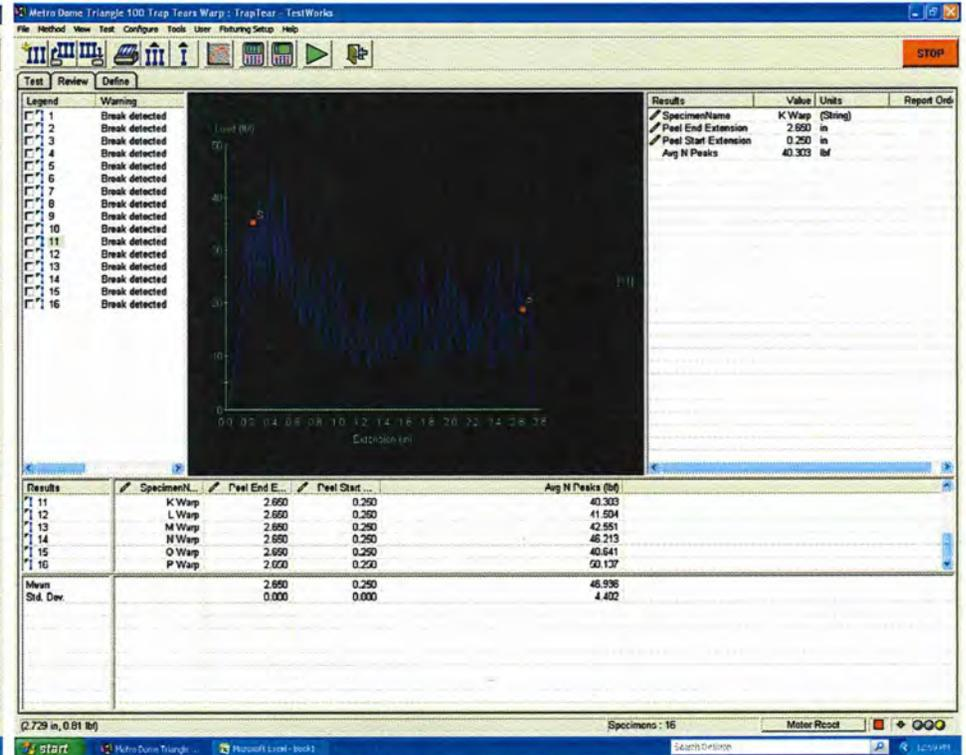
Figure 9: Panel 100 Trap Tear Sample K Warp Details
