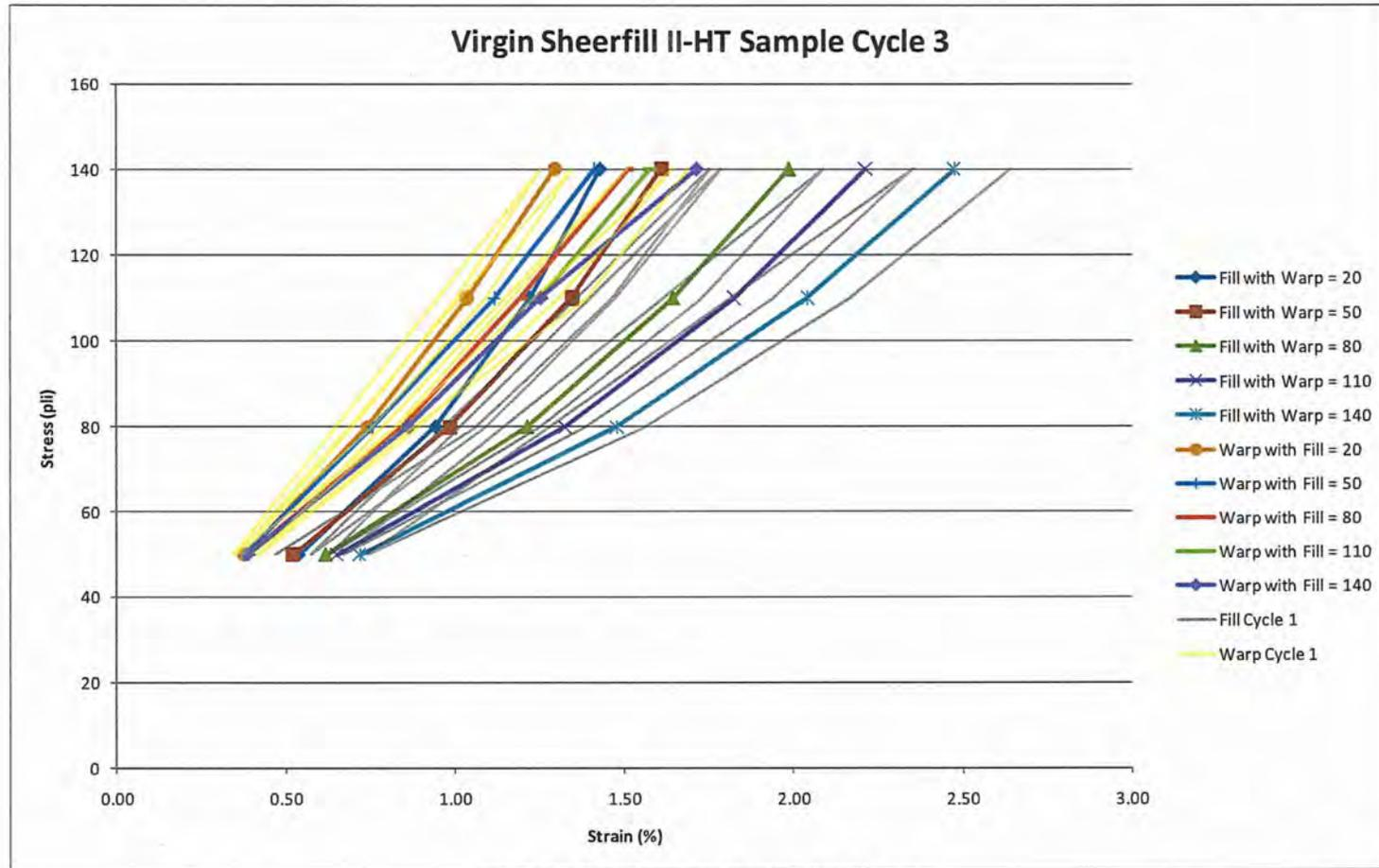
Figure 20: Virgin Biaxial Sample High Load Modulus Test Cycle 3
