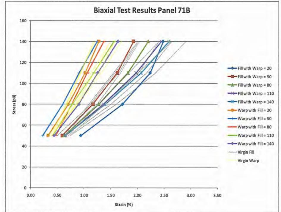
Figure 15: Panel 71B Biaxial Test Results
