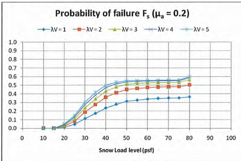
Figure 4 Probability of diamond panel failure under snow load, mean flaw size 12 mm
