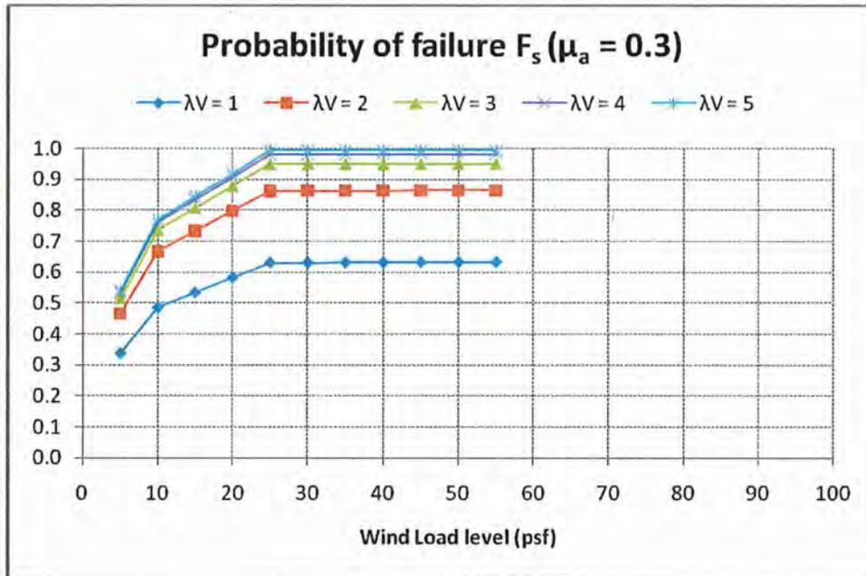
Figure 9 Probability of rectangular panel failure under wind load, mean flaw size 18 mm
