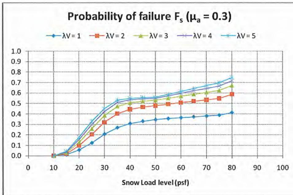
Figure 5 Probability of diamond panel failure under snow load, mean flaw size 18 mm
