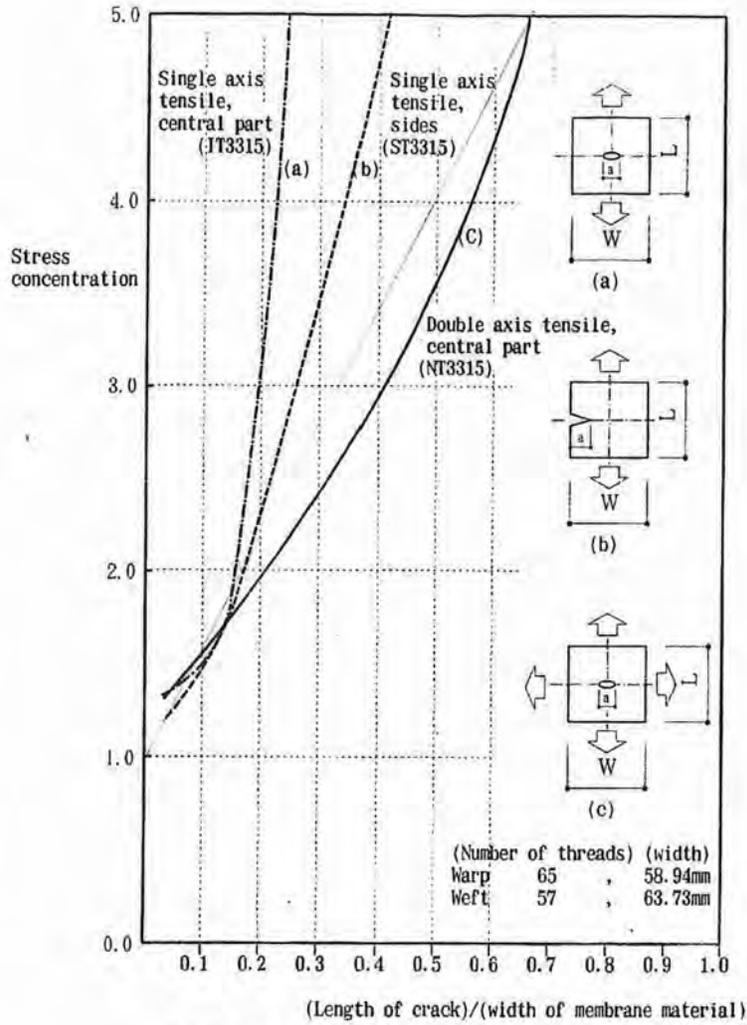
Fig.-15 Thread Loss Rate and Stress Concentration
