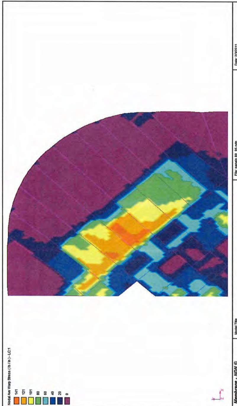
Figure 18 Panels 89-96 warp stresses
