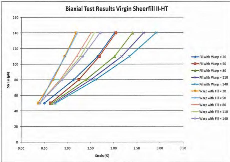
Figure 10: Virgin Sheerfill II-HT Biaxial Results
