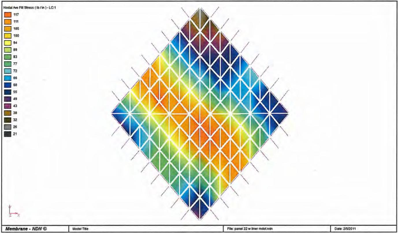
Figure 22 Panel 22 with liner fill stresses
