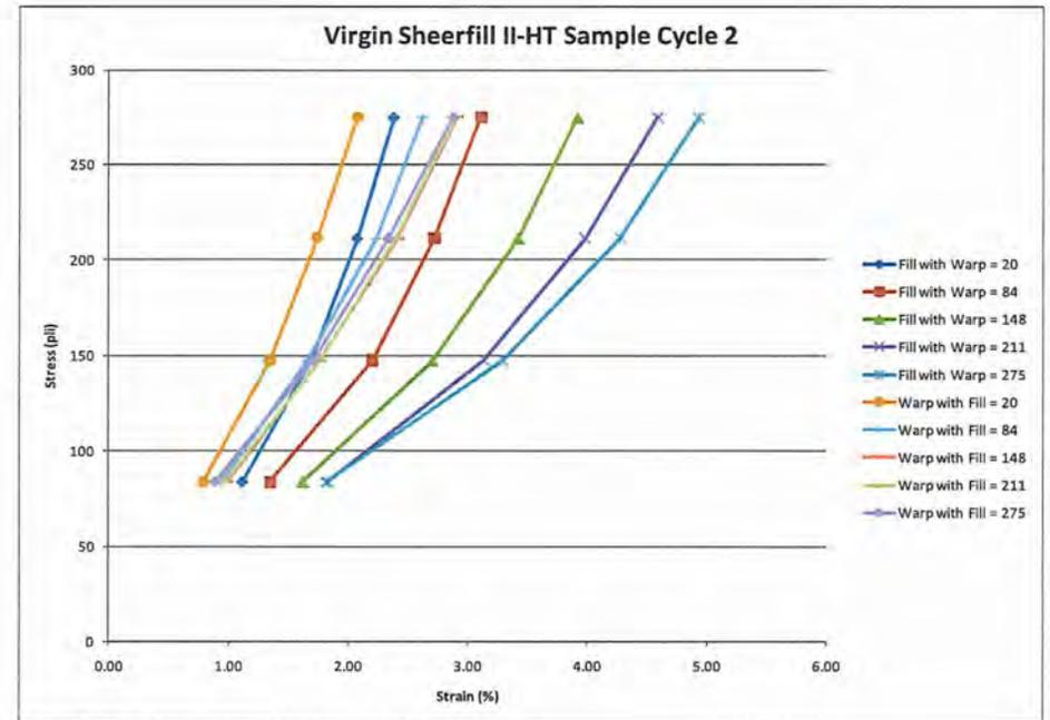
Figure 19: Virgin Biaxial Sample High Load Modulus Test Cycle 2
