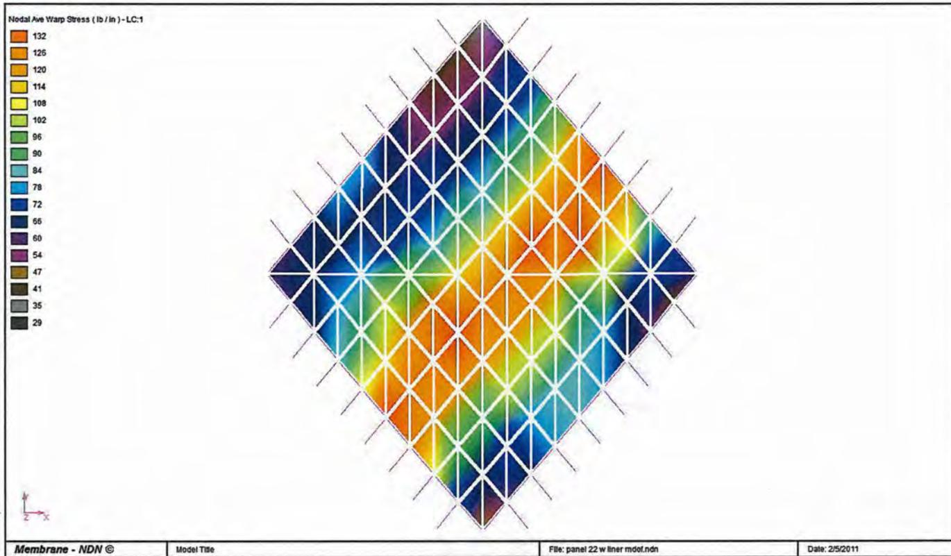
Figure 21 Panel 22 with liner warp stresses
