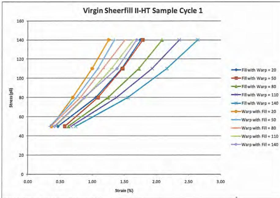
Figure 18: Virgin Biaxial Sample High Load Modulus Test Cycle 1
