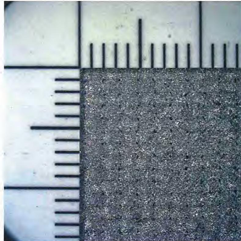
vertical spacing as 10 holes in 10.5mm = 1.05mm o.c.
