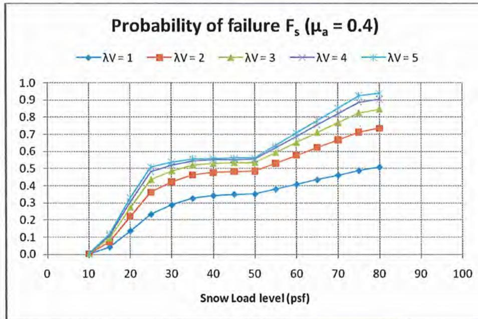
Figure 6 Probability of diamond panel failure under snow load, mean flaw size 24 mm
