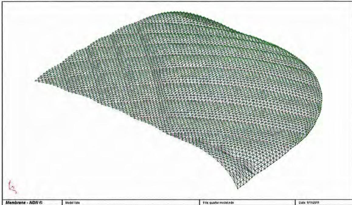
Figure 1: Roof Model Inflated
