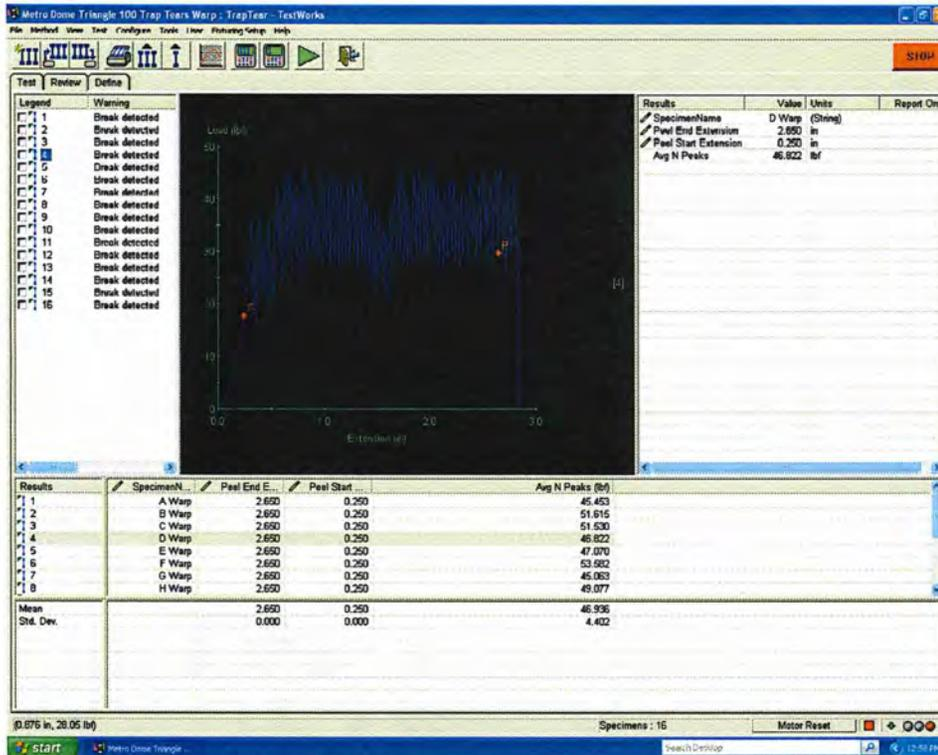
Figure 8: Panel 100 Trap Tear Sample D Warp Details
