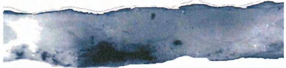
Figure 29: Cross Section of PTFE-Fiberglass Fabric from BC Place Showing Ink Penetration Test
