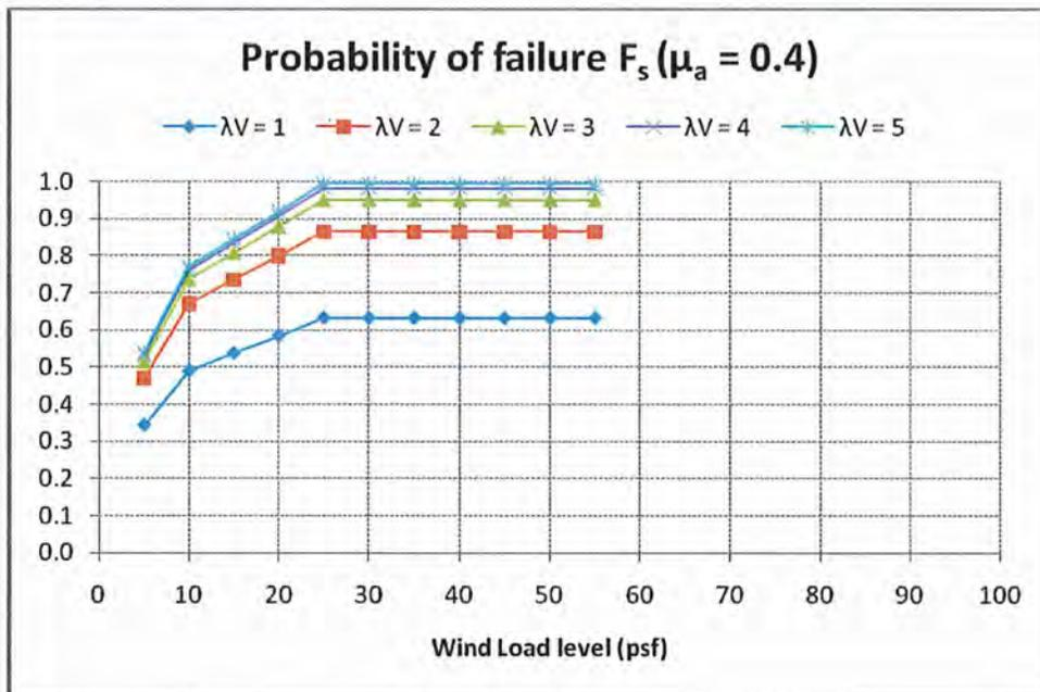
Figure 10 Probability of rectangular panel failure under wind load, mean flaw size 24 mm
