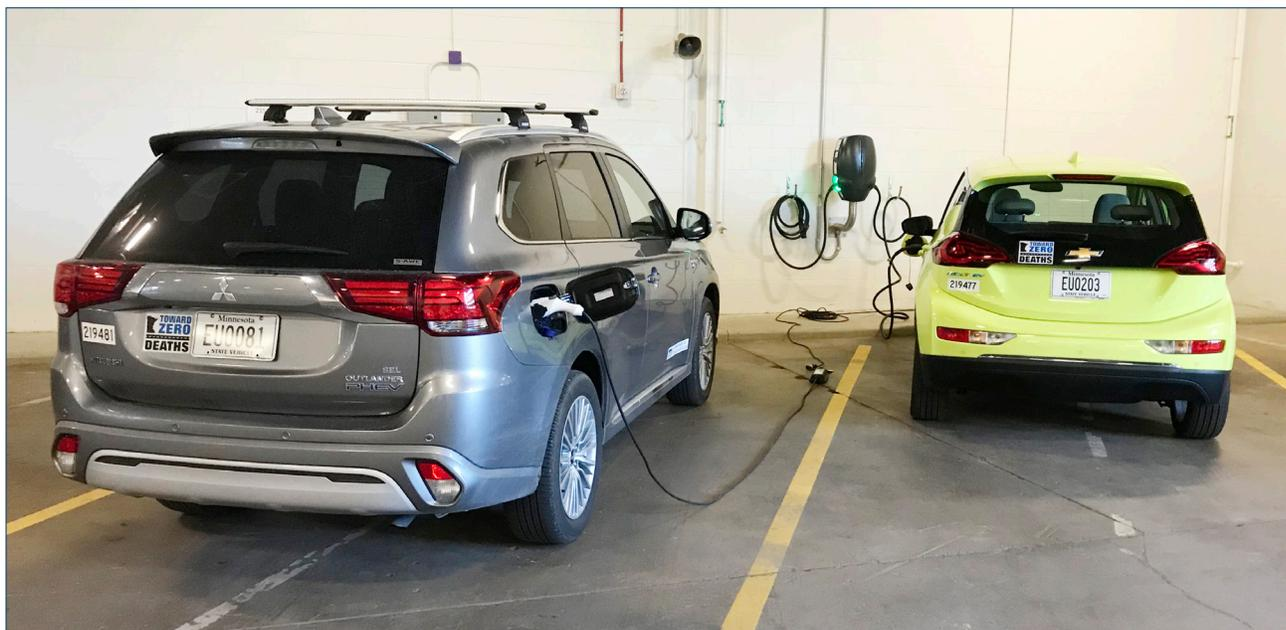
📷 A plug-in hybrid electric vehicle and a battery electric vehicle charge in a motor pool garage
