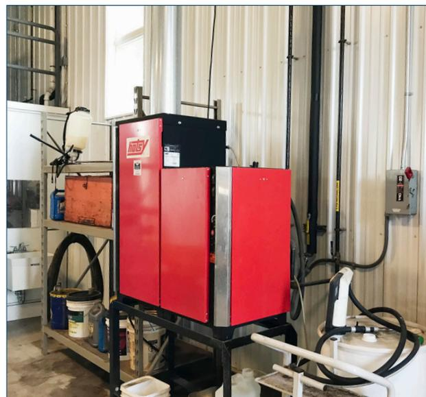
📷 A hot water pressure washer used to reduce water use when washing equipment
