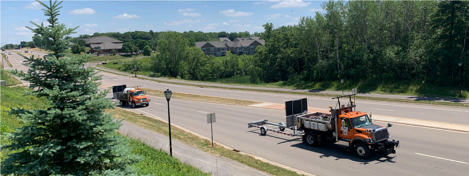
Autonomous Truck Mounted Attenuator system on road
