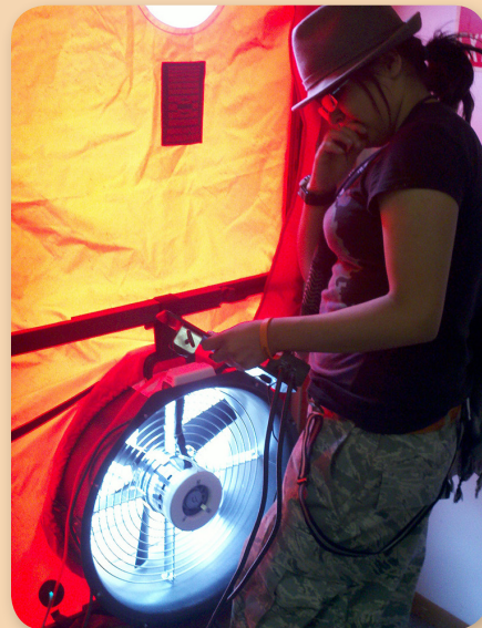
Miranda analyzes a manometer during a blower-door test.
