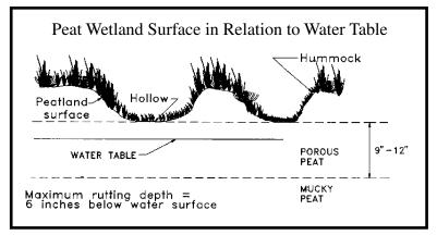
**Figure TH-10:** The water table (solid line) is near the bottom of the hollows (upper dotted line). Operations should stop when ruts reach 6 inches below the water table or 6 inches below the bottom of the hollows, whichever is lower. Peat is usually still porous 9 inches below the hollows, and ruts will heal in 2 to 3 years. Deep ruts (more than 12 inches below the hollows) will bring up well-decomposed, mucky peat and may take more than 20 years to heal.
