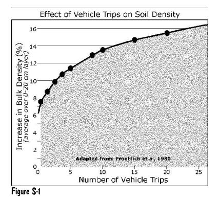
The first few trips (with heavy equipment) over the soil surface produce the greatest increase in soil density. A large percentage of the increase in soil density occurs during the first six trips on some soils (Froehlich et al 1980). (See Figure S-1.) Machine vibration may also contribute to compaction.
