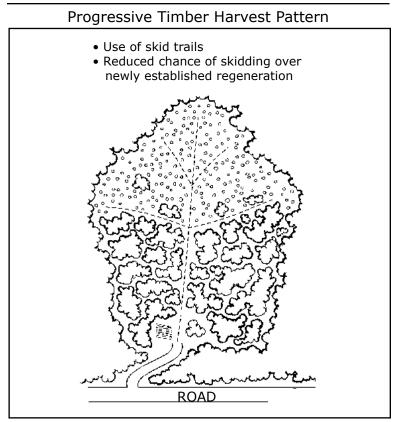
✓ Plan a progressive harvesting technique that avoids trafficking over pre-cut areas where possible. See Figure TH-2. For example, back-to-front harvesting techniques in frozen and unfrozen conditions can reduce site impacts during harvesting. Advantages of this method include the following:
