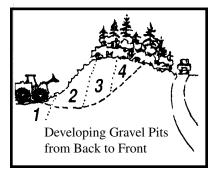
**Figure ROAD-6:** Develop gravel pits from back to front, moving toward predominant viewer or vantage point. In this illustration, Stage 1 has been completed, Stage 2 is in process, and Stages 3 and 4 will follow. Leaving the area adjacent to the road beyond Stage 4 untouched could result in no negative visual impact on the travel route.
