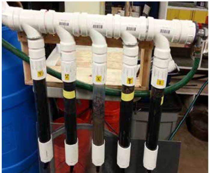
The picture above shows the column experiment system used in the study to examine the performance of the treatment technology using real stormwater. This picture was taken at the St. Anthony Falls Laboratory at the University of Minnesota.
