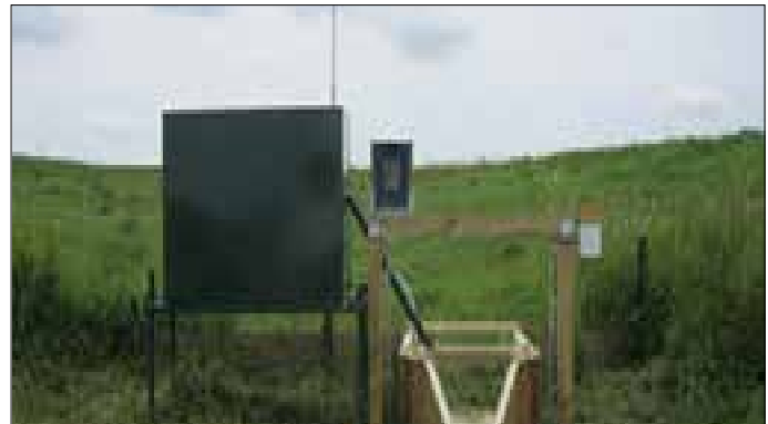
Monitoring site facing upslope. The H-flume and instrument shelter are visible.
