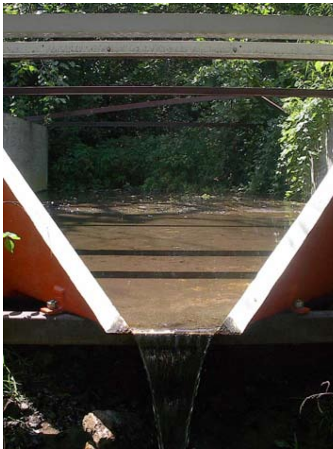
HL flume used to measure flow at paired-watershed monitoring sites, Whitewater River Watershed NMP Project, near St. Charles, MN.
