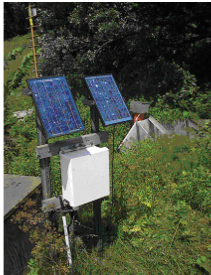
Weir and automated data logger on one of the paired field studies.
