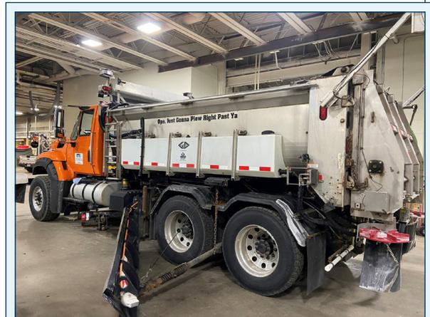
*📷 The Moorhead Truck Station snow plow truck has the capacity to carry approximately 2800 gallons of salt brine distributed between the side saddle tanks, an inbox storage tank and tanks mounted on the tow plow it pulls behind it.*
