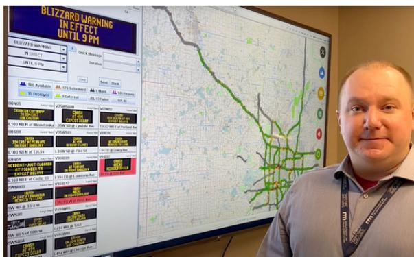
*Real-time weather alerts can be automatically posted to DMS through MnDOT's new system.*
