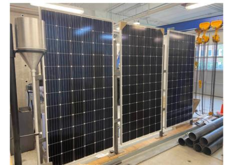
*The research team developed a prototype photovoltaic noise barrier system.*
