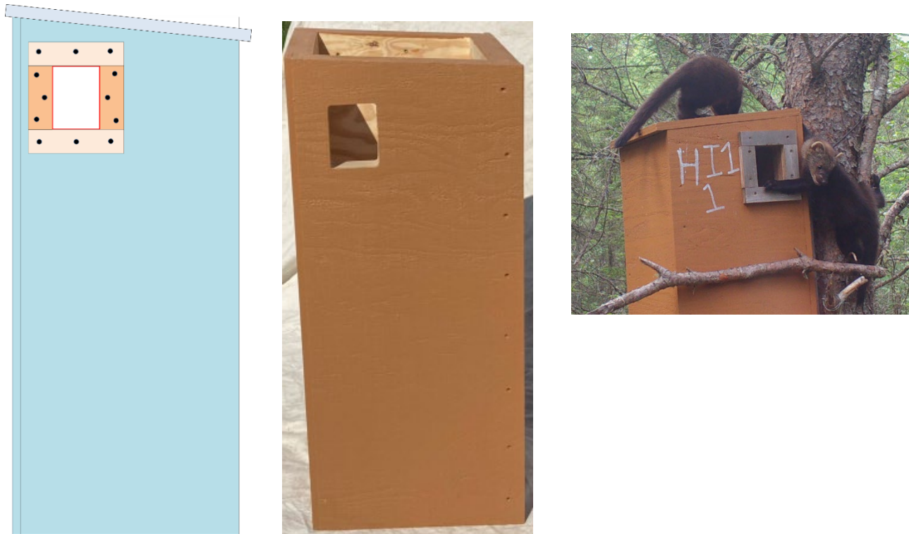
Figure 3. Side view of den box with opening, showing the additional 1x2 pieces that are screwed into the opening. An unfinished opening is shown in the middle picture, and fishers at a den box are shown in the right picture.
