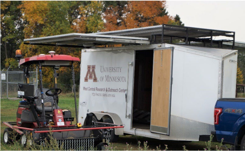
Cowbot Charging in Pasture with Solar Trailer
