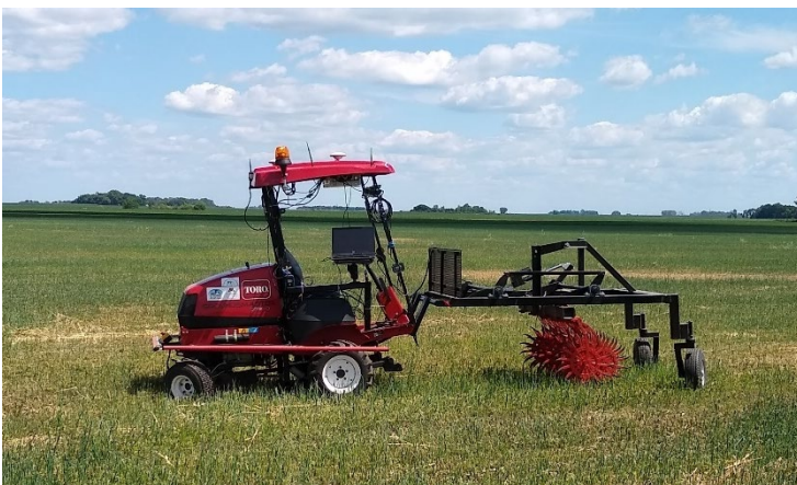
Cowbot Field Test with Rotary Hoe Weeding Implement Attached
