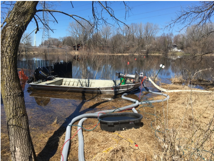
Figure 4. Boat with Whooshh transport system. Netted carp would be dumped into boat placed manually into transport system to be moved to water tanks with anesthetic.
