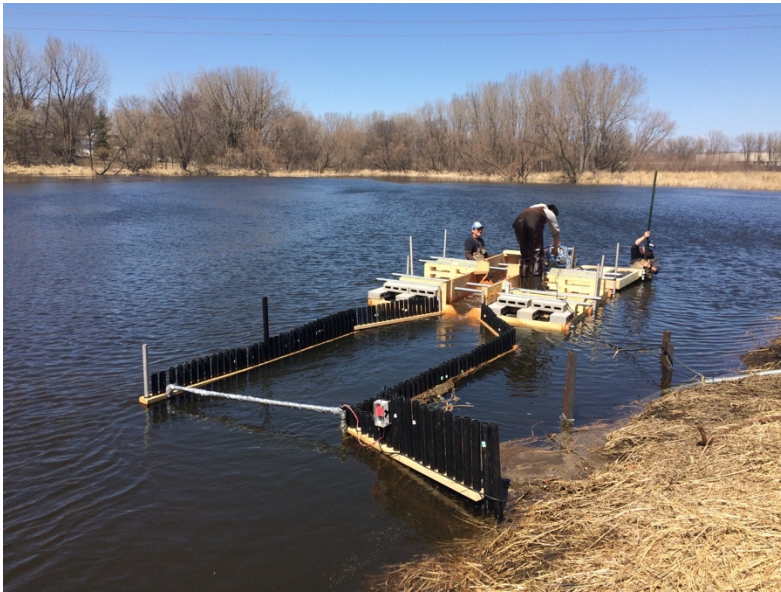
Figure 3. A PVC fence was used to guide carp into the ladder. An electric guidance system (EGS) is stretched across the stream to the left of the fence. Carp that migrate upstream are deflected by EGS and directed into the fence, floating carp ladder, and then Whooshh. For more details of the field design see Activity 1.
