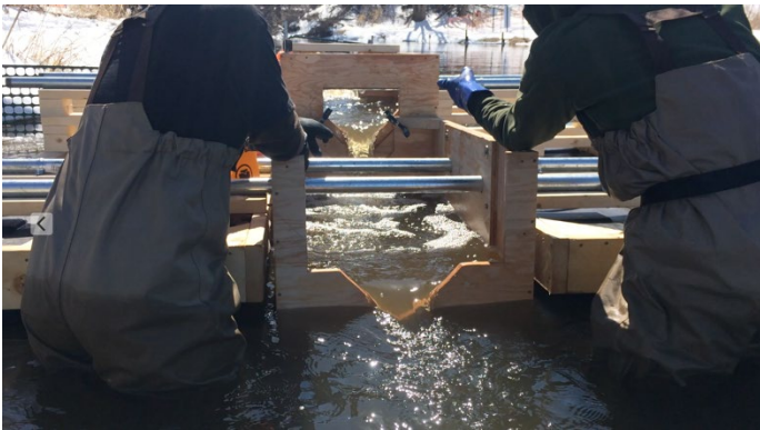
Figure 2. Downstream view of the carp ladder. The entrance to the ladder is at stream level and the water level increases by ~ 5-10 cm at each step of the ladder. Water pump was attached to the ladder exit to pump water through it.
