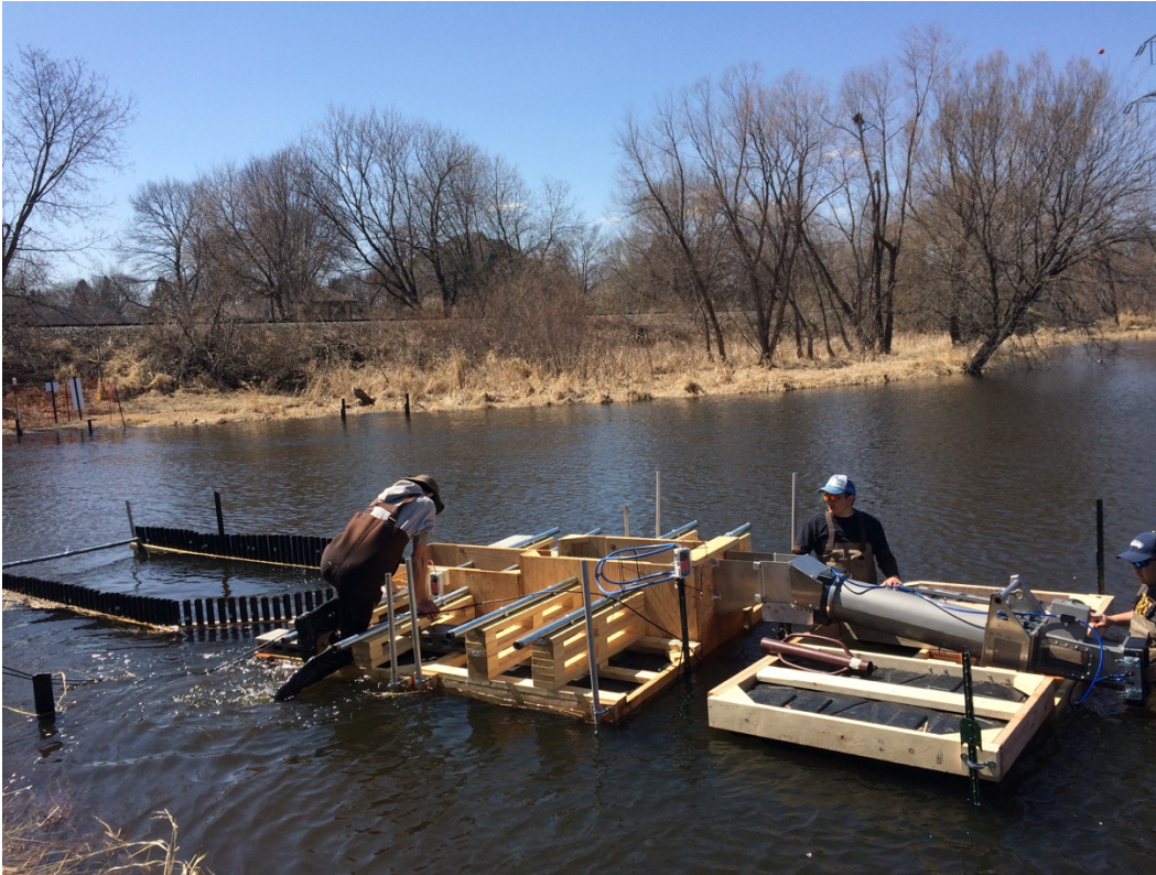
Figure 1. Carp ladder (plywood boxes) attached to the entrance to Whooshh. Note that the entrance to whooshh is ~ 25 cm above the surface of the stream, thus, the exit from the ladder had to be at the same level.
