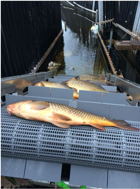
Figure 3. Conveyor used to remove carp from the stream.
