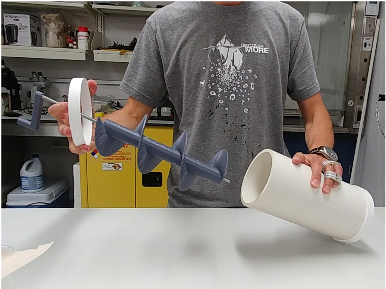
Figure 3. 3D printed auger mounted in PVC pipe, with hand crank. Motor powered spinning was achieved by removing hand crank and directly attaching drill to bolt.
