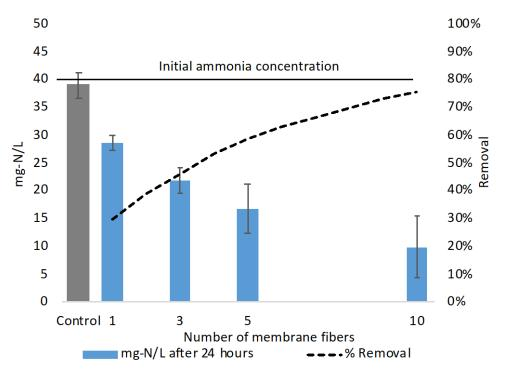
Figure 1.1. Ammonia removal from synthetic wastewater with zeolite coated alumina hollow fibers
