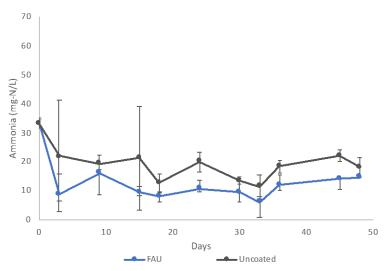
Figure 1.2. Ammonia effluent concentrations from biologically active batch reactors with zeolite-coated (labeled "FAU" for faujasite-type zeolites) and uncoated alumina hollow fibers. It can be seen that the faujasite-coated fibers removed more ammonia than the uncoated fibers over the course of the experiment.
