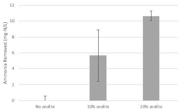
Figure 1.3. Ammonia removal after 24 hours by sorption to carriers containing different quantities of zeolite on their surface (no zeolite, 10% zeolite by mass, and 20% zeolite by mass).
