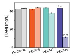
Figure 1.6. Ammonium removal from 45 mg/L ammonium solutions after 24 hours. The carrier labeled "PEX480" contained no zeolite. The carrier labeled "PEZ441" contained a low quantity of zeolite and the carrier labeled "PEZ444" contained 45% by mass zeolite. The concentrations shown represent the average of three separate experiments, with the error bars representing the standard deviation.
