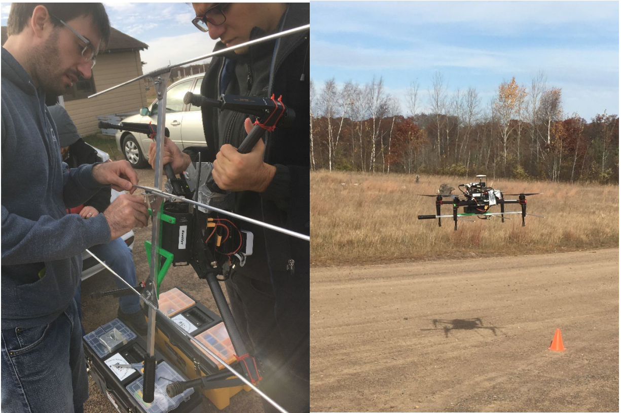
Images 1A (left) and 1B (right): 1A-Development of a custom-made UAV for the tracking of VHF signals utilizing a traditional wildlife Yagi. 1B-Testing the VHF-homing UAV at Cedar Creek Ecosystem Science Reserve. We placed VHF transmitters throughout the area and tested the ability of the UAV to detect, collect data, and search out the location of the transmitters.
