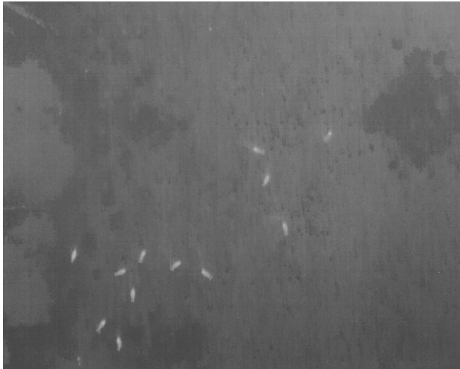
Image 4: Raw thermal imagery from a flight over a captive bison herd at the Cedar Creek Ecosystem Science Reserve. By collecting imagery in areas where we know the number of individuals present, we can improve on our understanding of detection and further refine field and analytical methods.
