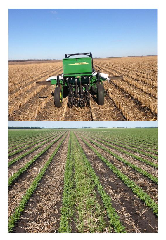
**Figure 1**. Upper : custom no-till seed drill designed to plant four rows in the 30 inch area between corn rows. Lower: Savanna grasses planted in November of 2016 and growing well between soy row planted in June of 2017.
