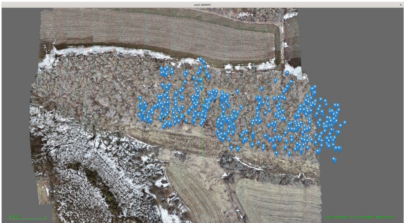
Photo by Curtis Olson, UMN, composite drone images of steep terrain in southeaster Minnesota after post processing via software Curt developed with ground truthed Oriental bittersweet points overlaid.
