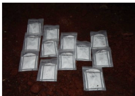
Fig. 1. In situ inoculation experiments with P. destructans . Packets are filled with sediment and inoculated with fungal conidia. Growth and reproduction of P. destructans will be monitored over two years.
