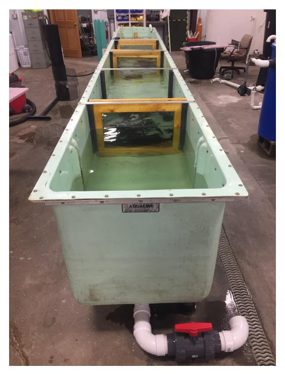
Figure 11. 30-foot flow through raceway, modified with compartments, used to hold host fishes such as Channel Catfish, Largemouth Bass, and Walleye.
