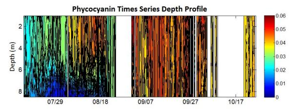
Figure 3. Phycocyanin measurements in Madison Lake, MN. The color legend indicates equivalent phycocyanin concentration in the lake. The y-axis is water depth starting at the lake surface, and the x-axis is time. The white rectangles (beginning of September and November) indicate periods when the profiler was not functioning to the excessive wind conditions above the lake surface.
