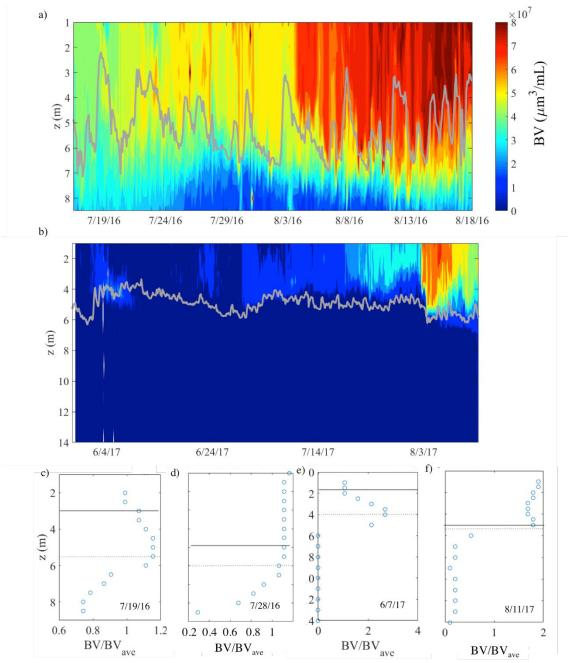
Figure. The temporal contour of BV water column profiles, where the gray line is the thermocline depth for a) Madison Lake and b) South Center Lake. c-f) Selected BV profiles from c,d) Madison Lake and e,f) South Center Lake. The dotted line is the thermocline depth, and the solid line is the depth of the diurnal surface layer.
