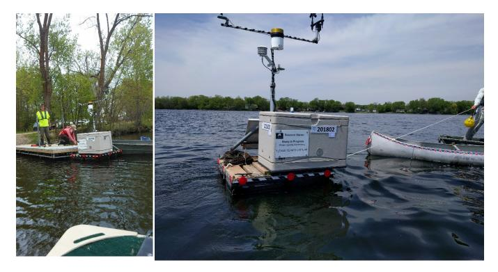
Figure. The cyanobacterial profiler with meteorological sensors, traversing stepper motor, and solar panel at the Ramsey Lake. The profiler was deployed on May 17<sup>th</sup>, 2018.
