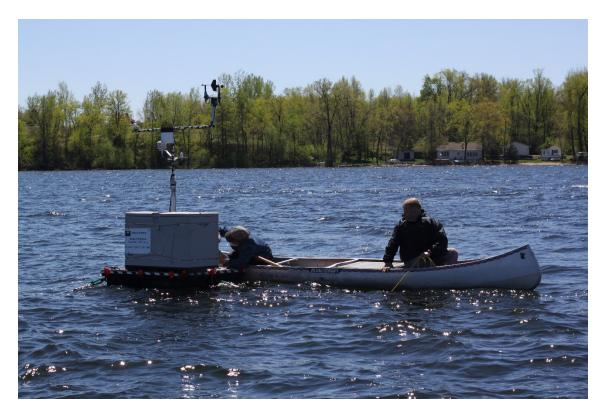
Figure. The cyanobacterial profiler with meteorological sensors, traversing stepper motor, and solar panel at the South Center lake. The profiler was deployed on May 18<sup>th</sup>, 2017.
