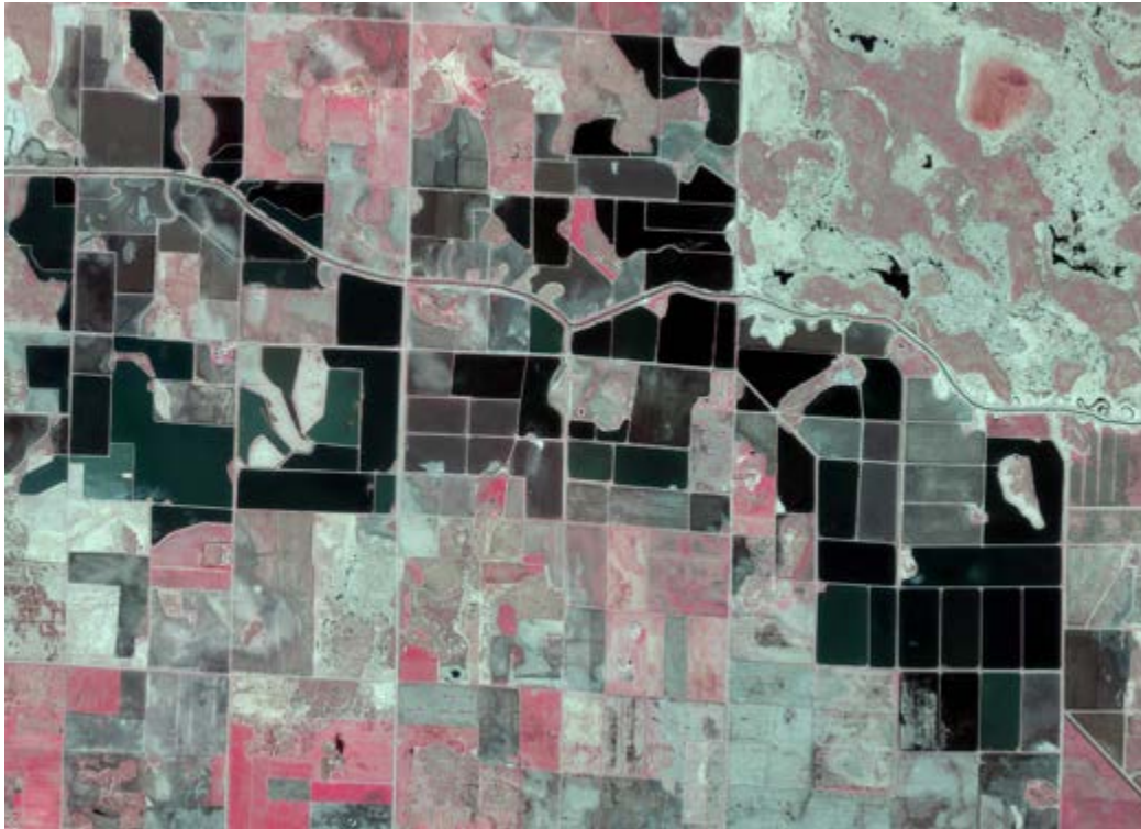
Figure 42. Wild rice plantation example, 2013/14 CIR; note unnatural shapes and black or dark blue (flooded) color.
