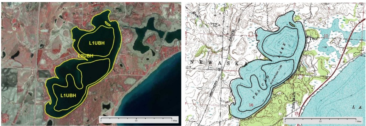
Figure 11. Lake contours on the DRG can help in determining the L1/L2 boundaries.
