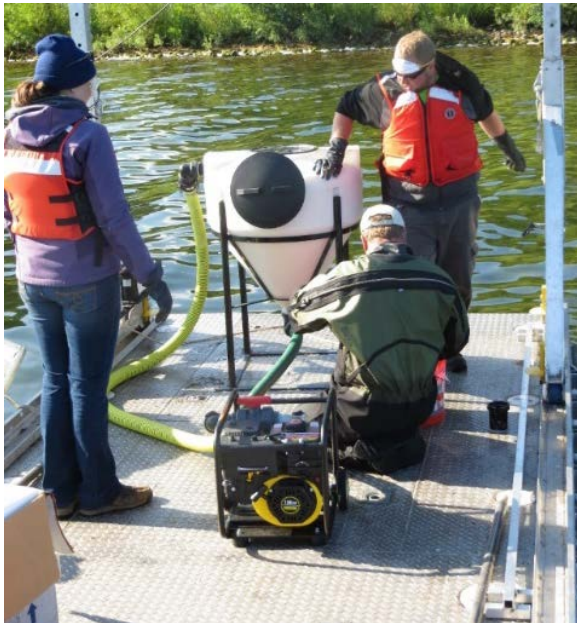
Figure 5. Zequanox suspension mixing system that was used to prepare the 5% (w/v) Zequanox suspensions for application to test enclosures in Robinson's Bay, Lake Minnetonka, MN.
