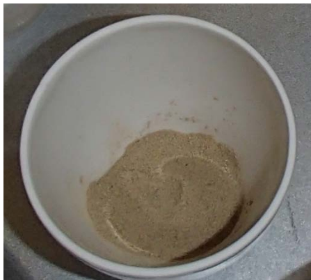
Figure 9. Dried and pulverized zebra mussel subsample in a crucible prior to burning in muffle furnace for determining zebra mussel biomass.
