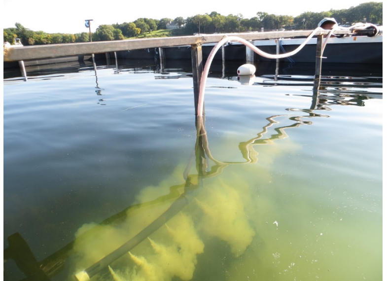
Figure 7. An application bar being used to apply Zequanox to a subsurface application enclosure in Robinson's Bay, Lake Minnetonka, MN.
