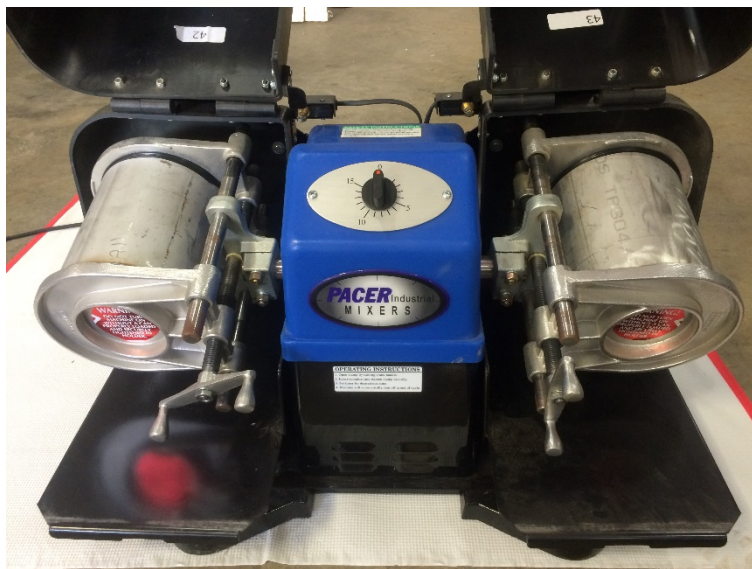
Figure 8. Industrial mixer with custom stainless steel containers used to pulverize dried zebra mussels prior to burning in a muffle furnace for zebra mussel biomass determination.
