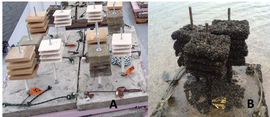
Figure 2. Example of multiple-plate (type 1) samplers before (A, Left) and after deployment for two growing seasons in Robinson's Bay, Lake Minnetonka, MN (B, right).
