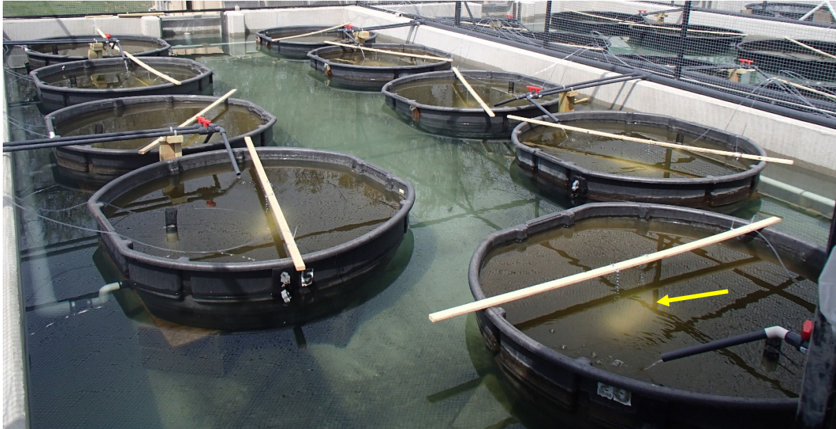
Figure 1. Test system in outdoor concrete ponds. Two ponds held nine 1000-L tanks in a thermal water jacket. Water was supplied to test tanks from an adjacent earthen pond. Amphipod test chambers (arrow) were suspended in the test tank at mid-depth. Mayfly chambers (not visible) were placed on the tank bottom. Each pond contained three replicates of each treatment (0, 50, and 100 mg/L A.I. Zequanox).
