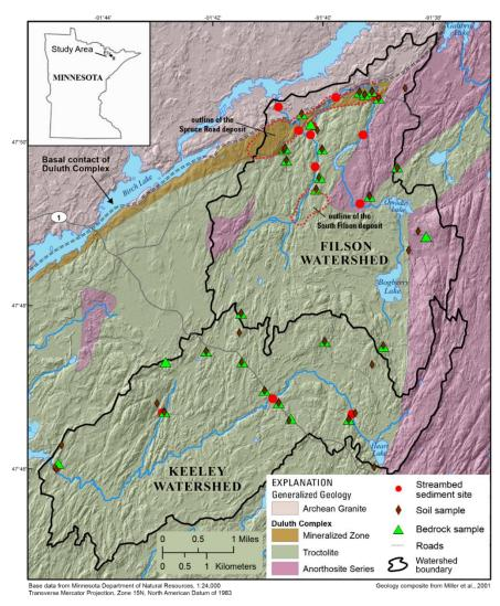
Fig 1. Solid media sample locations and bedrock geology along Filson Creek and Keeley Creek near Ely, MN.
