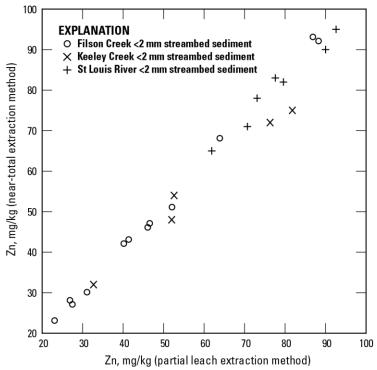
Fig 5. Concentrations of Zn in <2 mm streambed sediments from a partial leach extraction method that mobilizes only the soluble portion of the metal and from a near-total extraction that extracts all Zn in the sediment. Good correlation indicates that all Zn is soluble, likely sorbed onto Fe-Mn-oxy-hydroxides.
