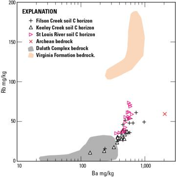
Fig. 3. Concentrations of Ba versus Rb (plotted on a log scale) for bedrok and soil C horizon samples from the three study watersheds. The gray field represents Duluth complex bedrock, the orange field represents bedrock of the Virginia Formation, and the red cross is the single sample of Archean granite. Soil from northern part of the Filson watershed trend towards the granite point; soil from the western St. Louis watershed trend towards the Virginia Formation field.
