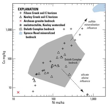
Fig 4. Concentrations of Ni versus Cu (plotted on a log scale) 16for bedrock and soil from Filson and Keeley watersheds. Soil collected within the mineralized zone have Ni and Cu values that trend towards mineralized bedrock (blue field); some soil in the Keeley watershed have Ni values that trend towards olivine-bearing, Ni-rich/Cu-poor melatroctolite (star).
