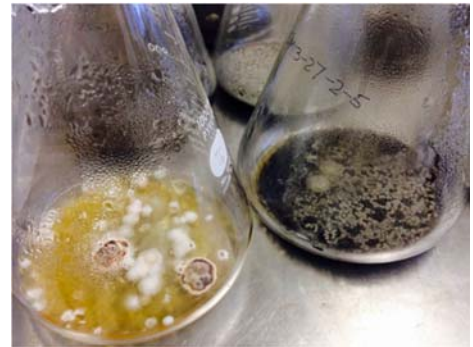
Figure 2. Fungi being grown in flasks with liquid media for heavy metal sequestration testing.
