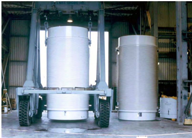
Loaded spent fuel storage cask on transporter is moved from the fuel handling building at the Surry Power Station in Surry, VA.
