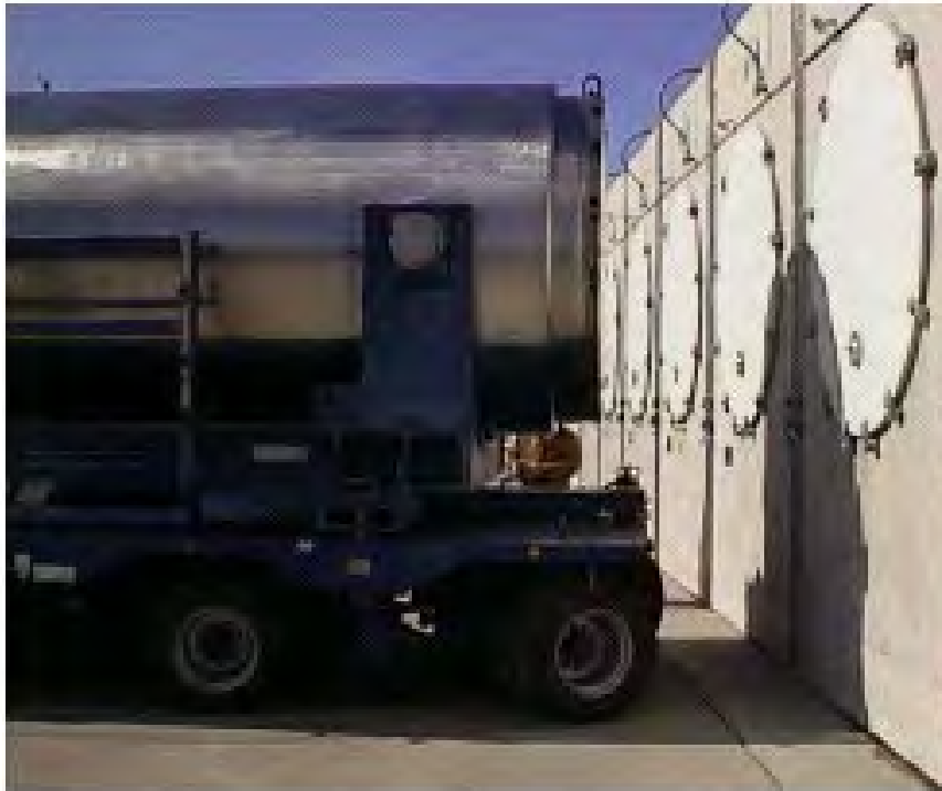
Figure C-4: Alignment of Transfer Cask with Storage Module
