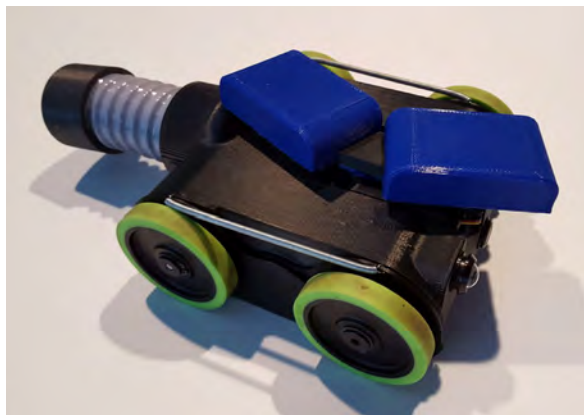
Prototype robotic delivery system. (Courtesy: EPRI/RTT)
