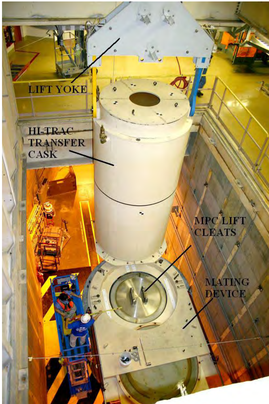
Figure C-10: Overpack, Mating Device, and Transfer Cask
