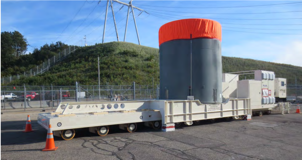
Figure C-9: Overpack on Crawler
