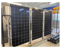
The research team developed a prototype photovoltaic noise barrier system.
