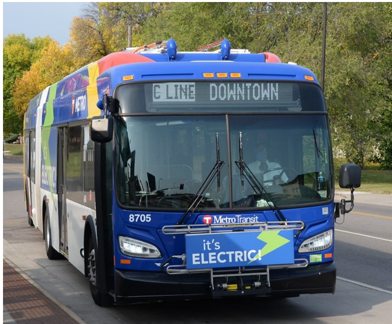
Figure 14 Metro Transit C Line 60-foot articulated BEB
