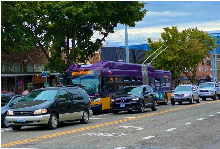
Figure 10 Trolleybus in operation with two trolley poles in Seattle, WA
