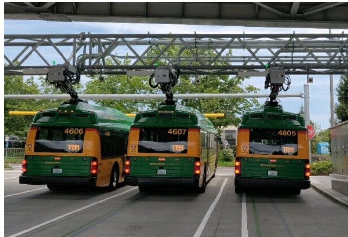
Figure 21: King County Metro overhead gantry charging system
