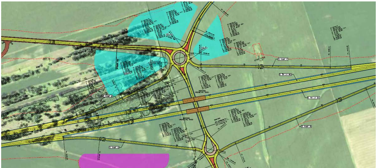
Figure 55a: Plan View of Hwy 14 – CR 12-24 Interchange
