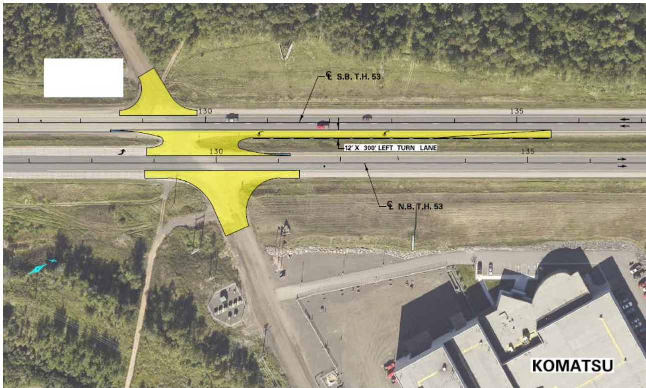
Figure 52: Plan View of Highway 53 at P&H Road
