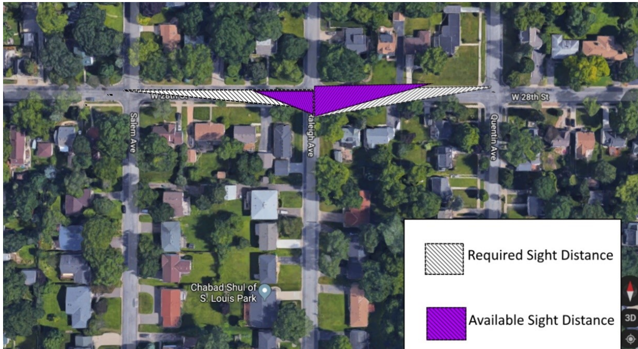
Figure 3.100 Available sight distance and required sight distance at Raleigh Ave and W 28 th St NB
