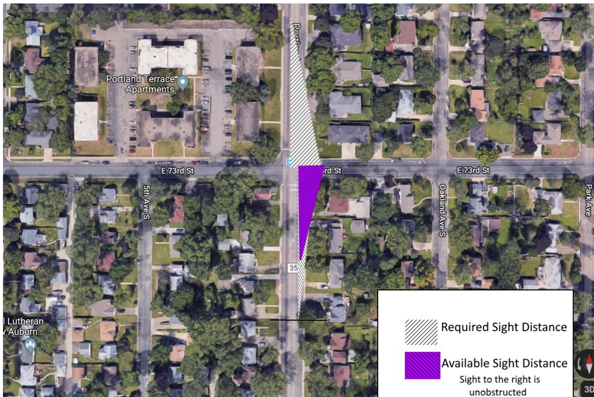
Figure 3.76 Available sight distance and required sight distance at Portland Ave and E 73rd St WB
