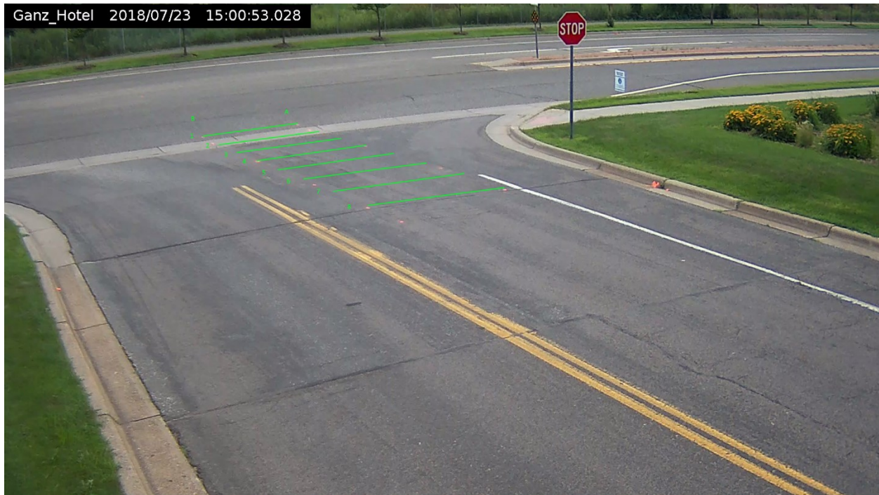
Figure 3.111 Camera view of the intersection of County Rd C W and Civic Center Dr with 5-ft overlay lines marked
