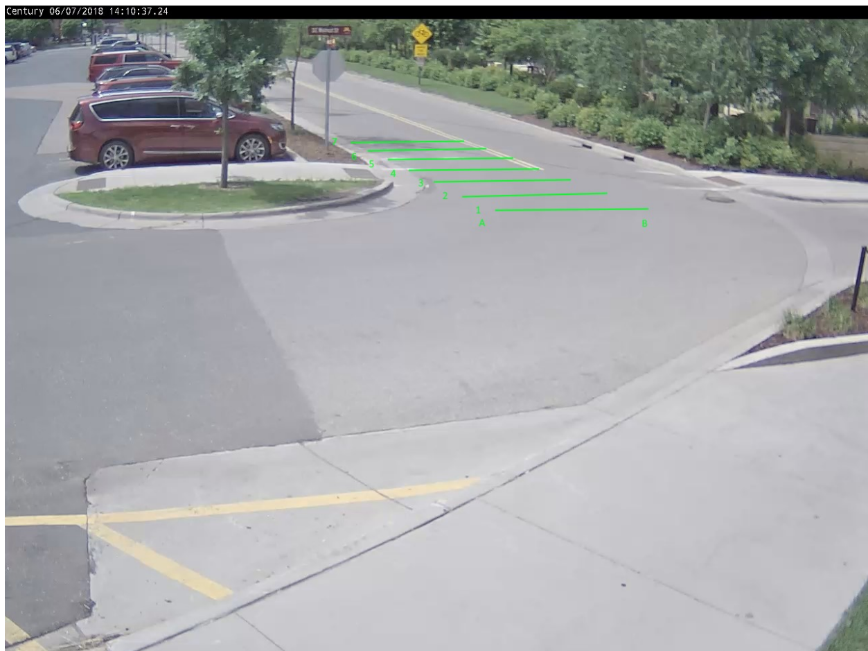
Figure 3.11 Camera view of the intersection of Walnut St SE and Beacon St SE with 5-ft overlay lines marked
