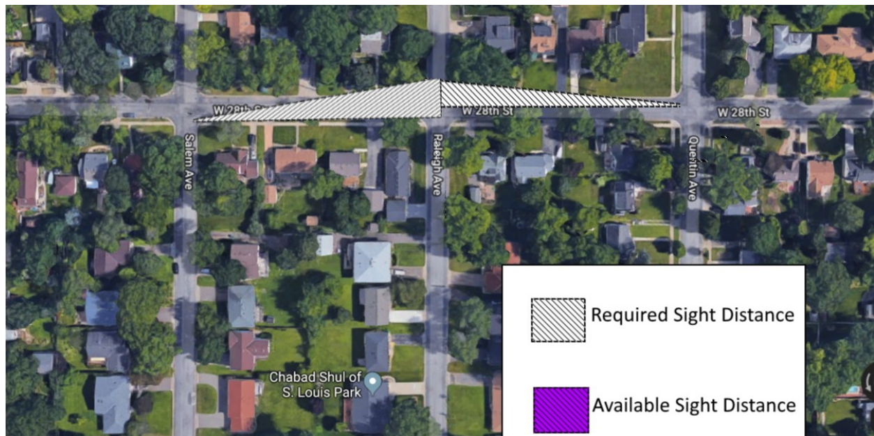
Figure 3.105 Available sight distance and required sight distance at Raleigh Ave and W 28 th St SB
