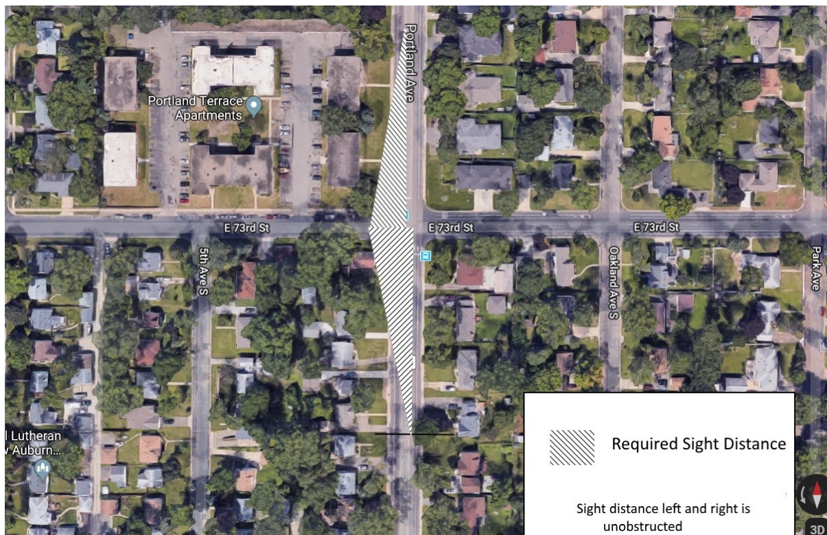
Figure 3.70 Available sight distance and required sight distance at Portland Ave EB
