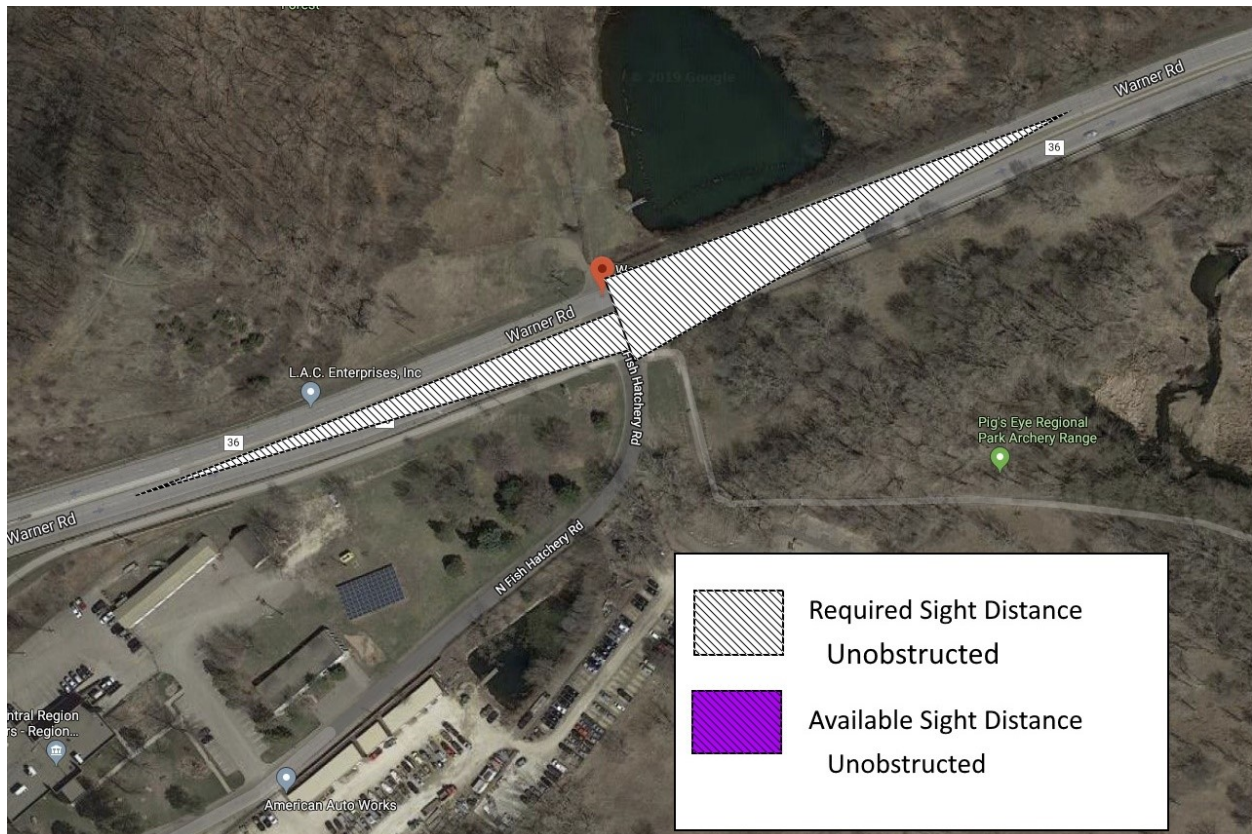
Figure 3.83 Available sight distance and required sight distance at Warner Rd and Fish Hatchery Rd N
