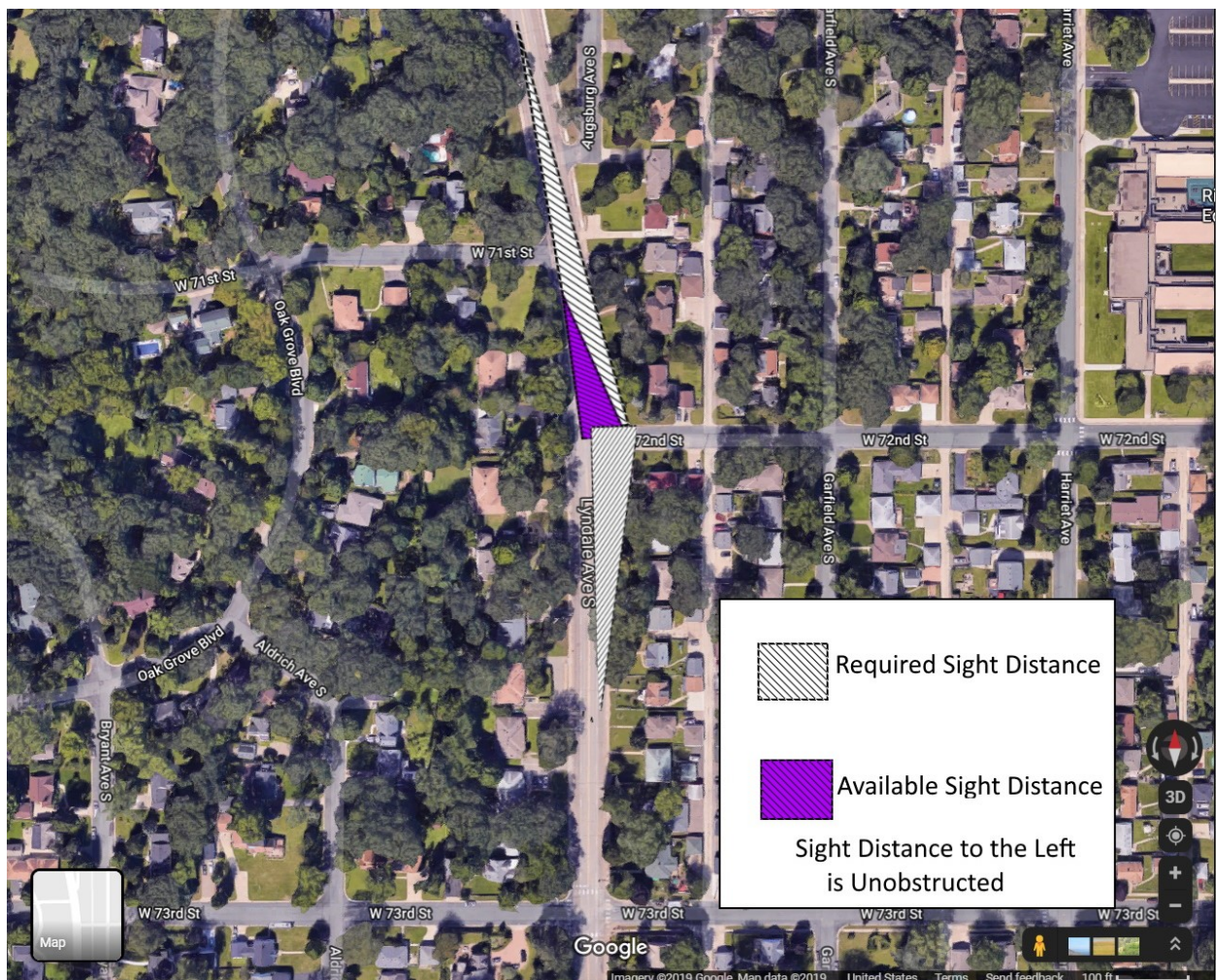
Figure 3.19 Available sight distance and required sight distance at Lyndale Ave S and W 72nd St
