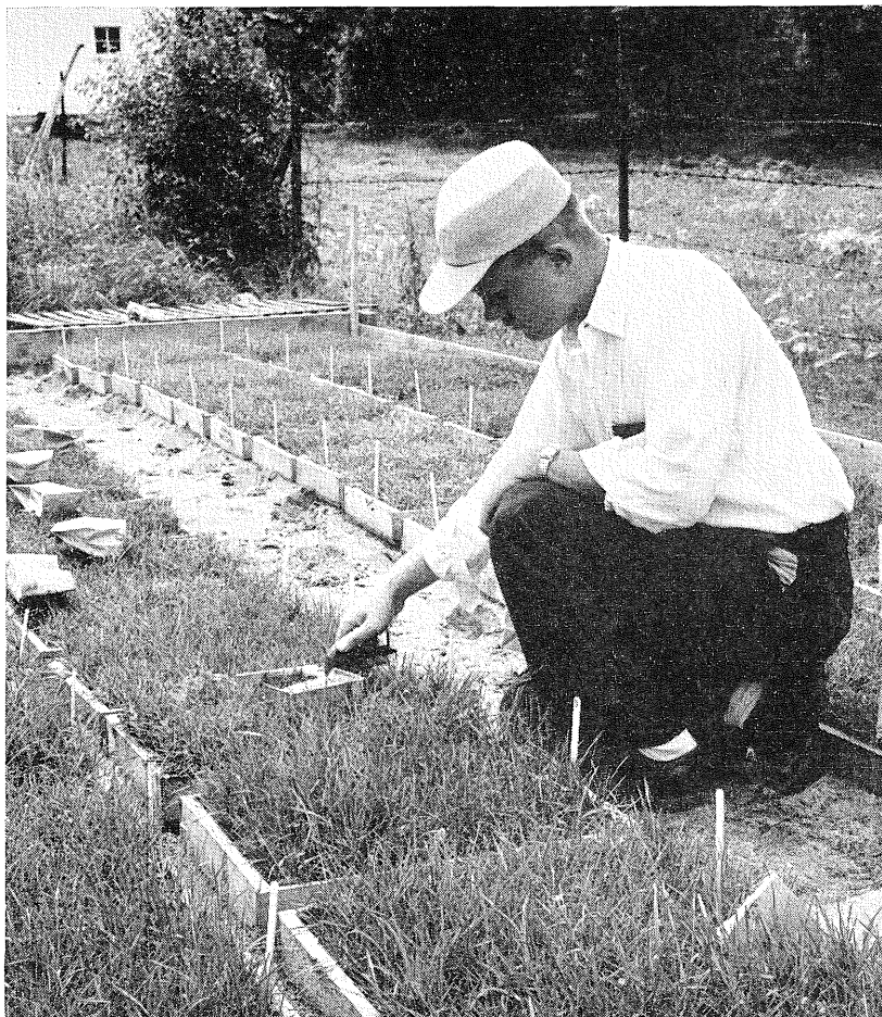
TURF TESTS of experimental peat products. Weight of clippings is key to product effectiveness. CPPP, soils and horticulture departments, St. Paul Campus, University of Minnesota (Figure 5).
