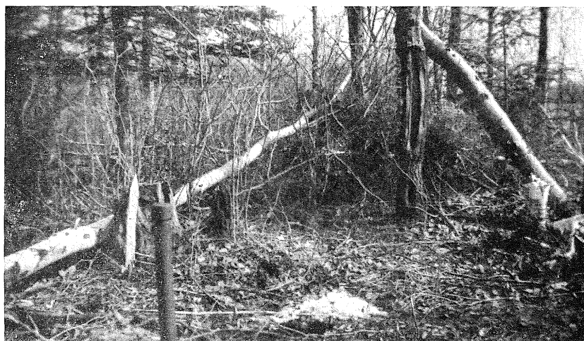
Decayed corner post is replaced by iron pipe with marked cap. At right in picture, note bearing tree in poor condition.
