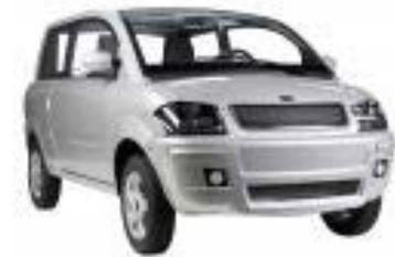
The electric vehicles are rechargeable through the electrical grid and normally have a range of 30 to 75 miles before needing to recharge. Models come in styles ranging from two-seaters to small-scale trucks, normally weighing between 1,000 and 1,500 pounds. Originally produced mostly for niche uses such as military bases and planned communities, their use has widened.
