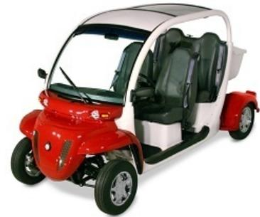
**Neighborhood electric vehicle.** Minnesota law defines a neighborhood electric vehicle (NEV) as a three- or four-wheeled, electrically powered motor vehicle that has a maximum speed of between 20 and 25 miles per hour on a flat surface. [Minn. Stat. § 169.011](#), subd. 47.
