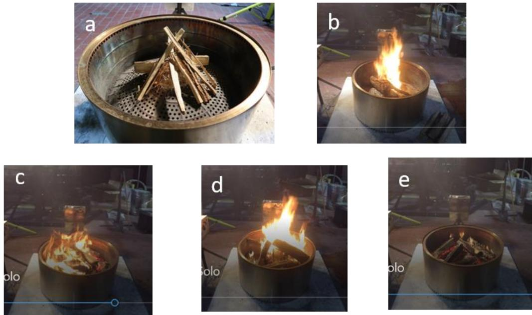
Figure 5. Burn phases of fire pit testing a) ignition fuel bed, b) ignition, c) burn-up phase, d) steady burn phase, and e) burn-down phase.
