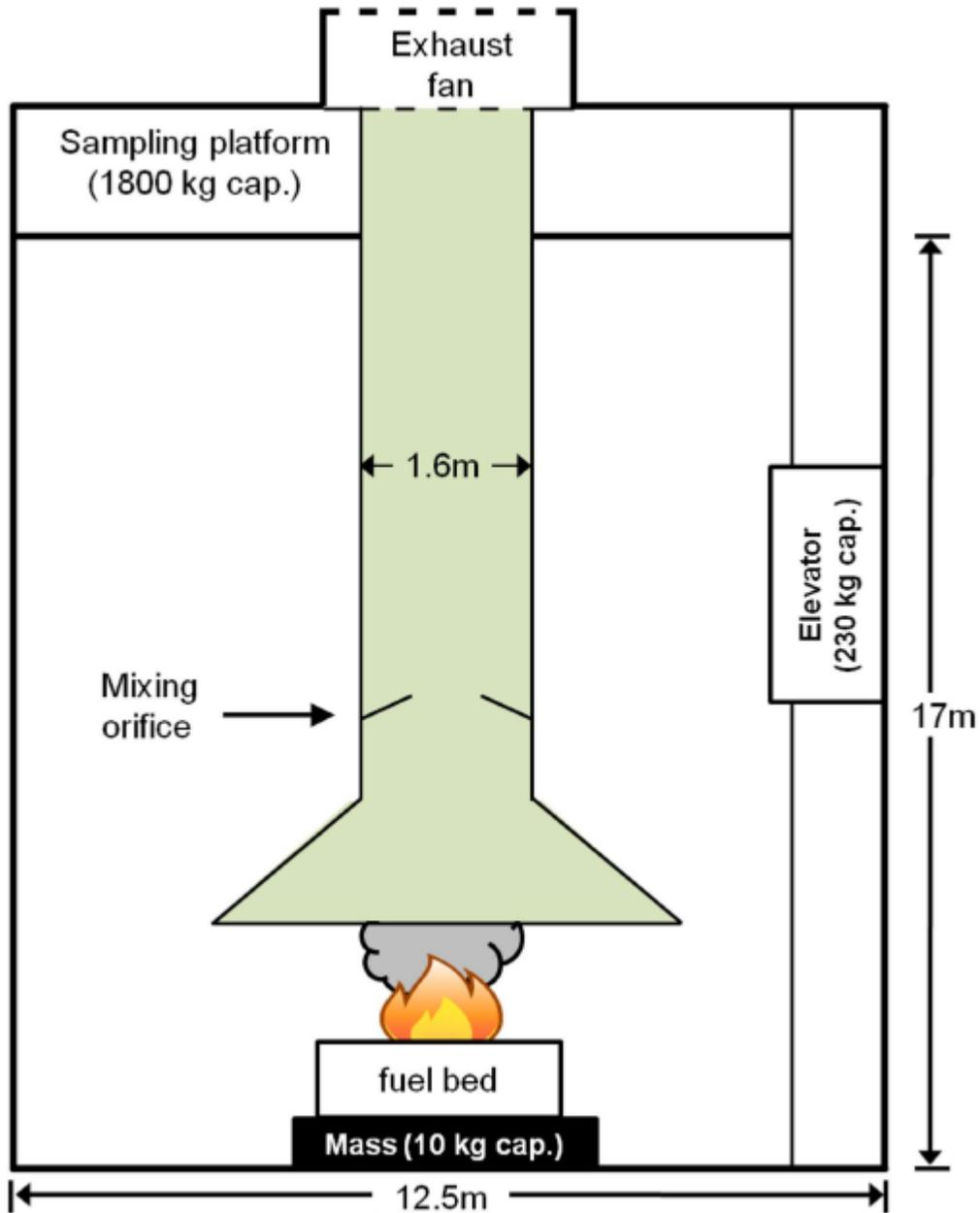
Figure 1. Schematic of combustion chamber at the Missoula Fire Sciences Laboratory (from Burling et al., 2010).
