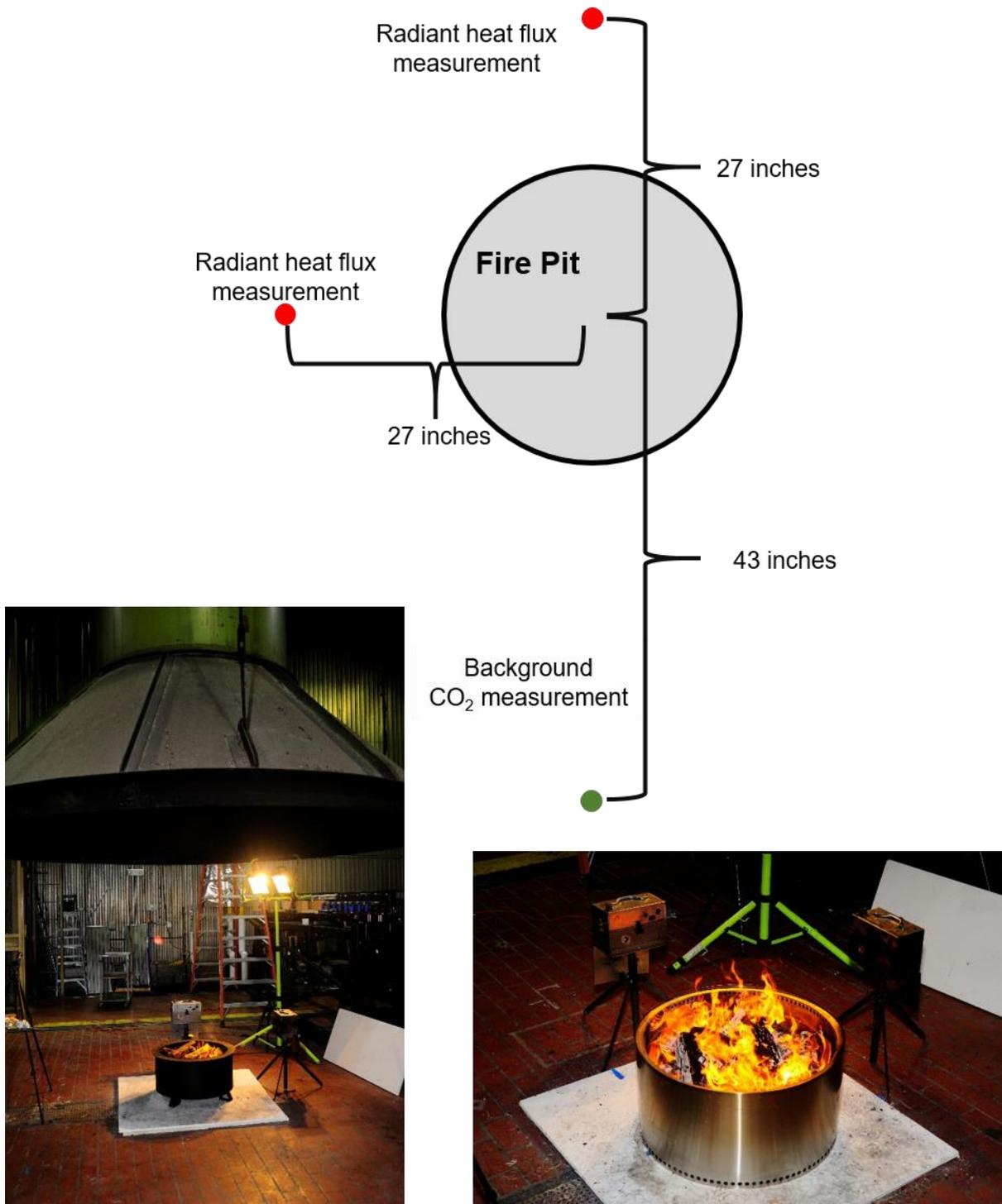
Figure 4. Schematic of experimental setup on the combustion chamber floor. The inset photo shows the position of the fire behavior packages containing the radiant heat flux sensors.
