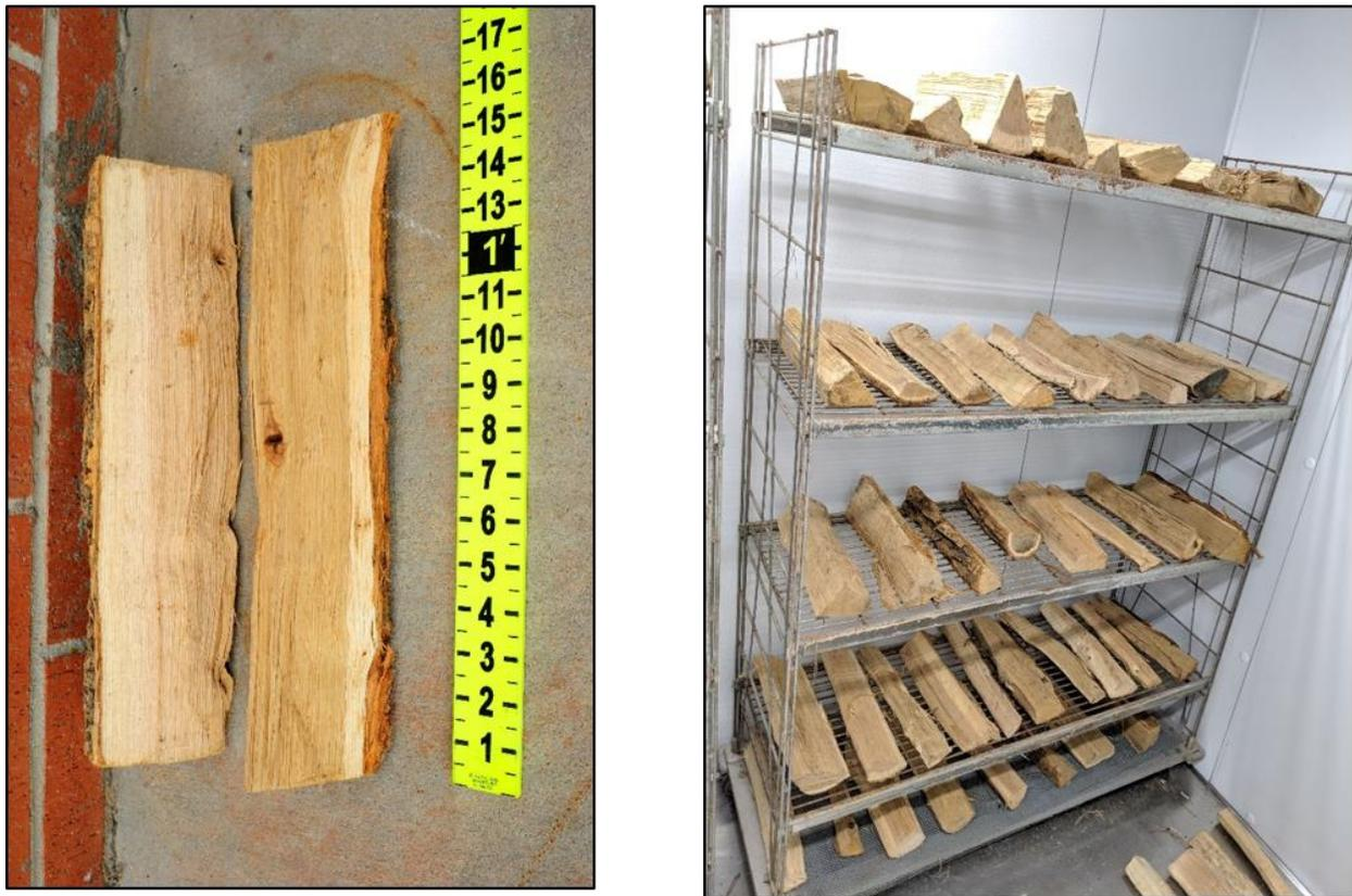
Figure 3. Left: Typical pieces of split firewood, right: firewood conditioning the environmental chamber at the Missoula Fire Sciences Laboratory.
