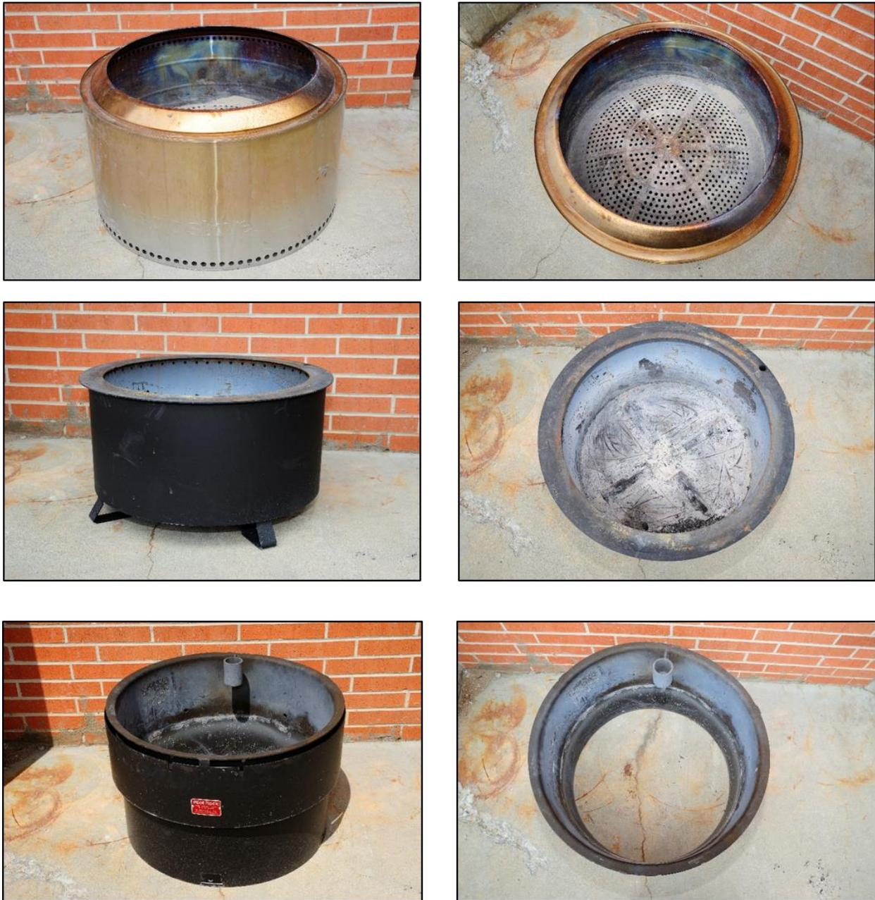
Figure 2. Fire pits post testing. Top row: Solo Yukon Stove, middle Row: Breeo, bottom row: Pilot Rock (traditional campground fire pit).
