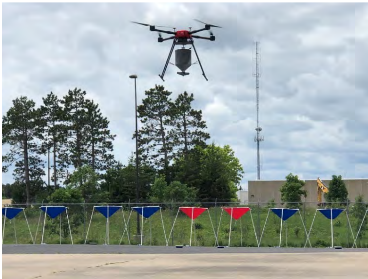
Figure 7.2 Calibrating PV-22 UAS + granular applicator.
