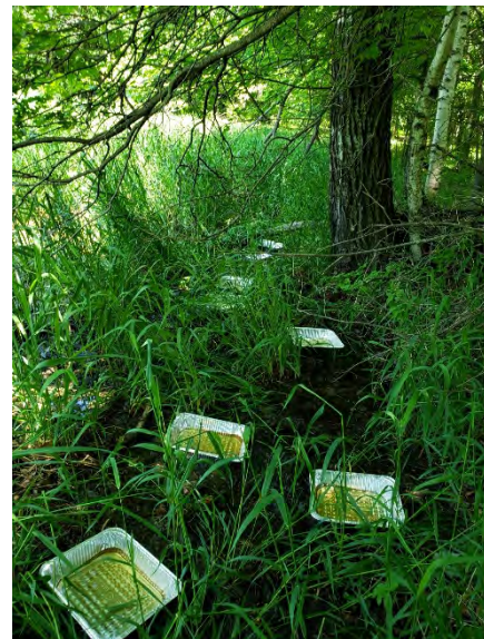
Figure 7.3 Testing granule deposition under tree canopy.
