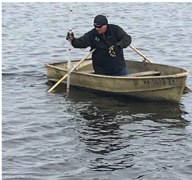
Figure 3. Frank Stuemke, a pond expert with MRWA, measures the sludge depth of a pond in Sandstone, Minnesota.
