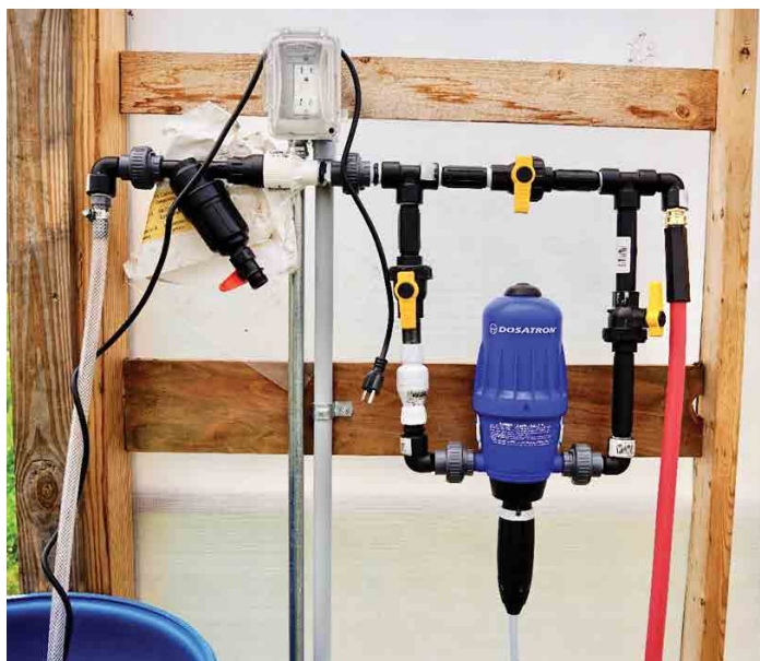
Dosatron assembly for fertigation at The Good Acre.
