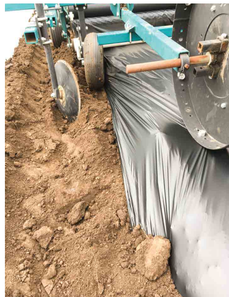
Bio360 biodegradable compostable black plastic mulch being installed on a 6 inch raised bed.
