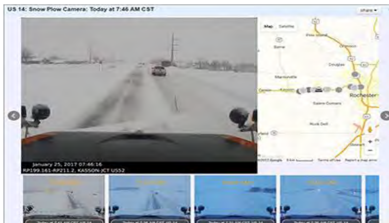
This is a screenshot of the 511 website showing the image from an active snow plow. The webpage shows the location of the plow, date, time and location. The film strip at the bottom shows where the plow has been every five minutes.
