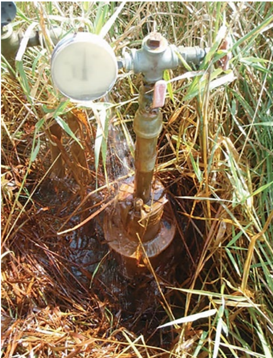
Photo 38: Monitoring well in need of replacement.
