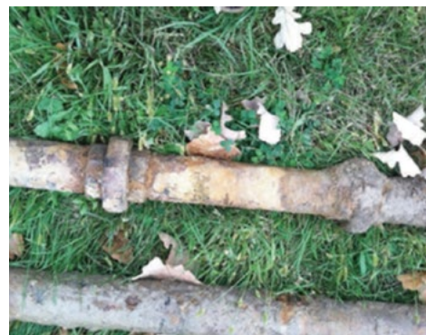
Photo 16: Itasca State Park—corroded steel water pipe.
