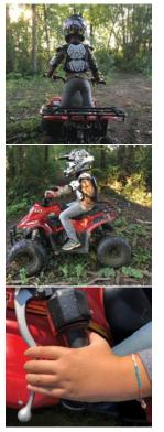
Seat clearance: There should be a minimum of 3 inches between operator and the ATV seat. Proper clearance enables the operator to maintain balance on the foot rests when riding over rough terrain. Maintaining balance prevents the operator from falling off or being thrown from the machine
