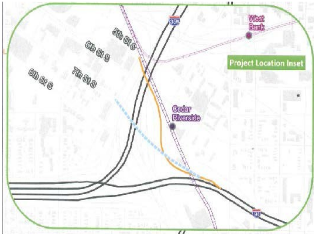
Figure 23: New 7th Street off-ramp and re-purposed 5th street off ramp at I-94
