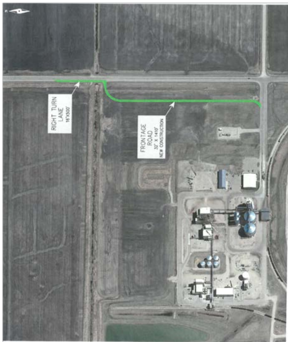
Figure 45: Plan View of Canola Oil Processing Plant Frontage Road
