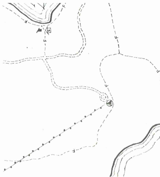
A January 1936 plan detail showing the tower (marked by a triangle) with foot trails ("F"), truck trails (double dashes), and a telephone line (line with dots) (Minnesota Dept. of Conservation Forestry Division Records, Minnesota Historical Society)
