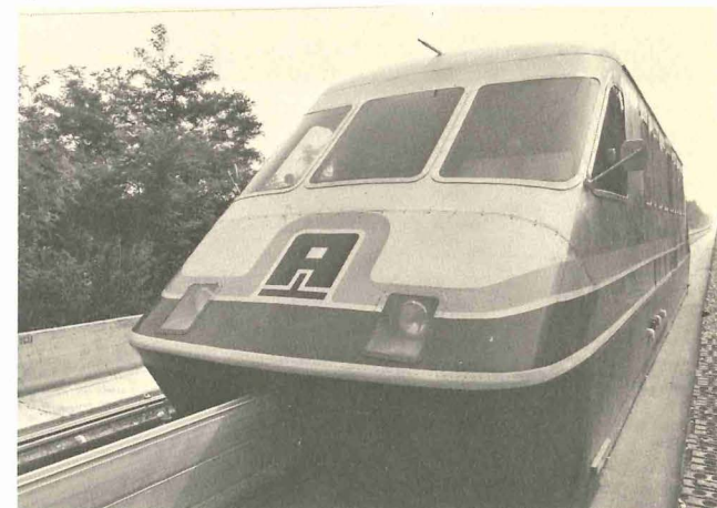
Tracked Air Cushion Vehicle With Linear Induction Motor
