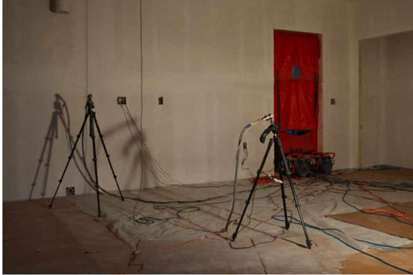
Figure 32. Example of aerosol sealing in a new construction application
