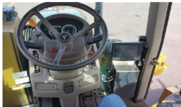
A metal rack (right) within the mower cab houses the AVL unit.
