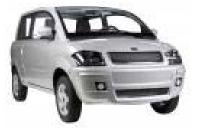
The electric vehicles are rechargeable through the electrical grid and normally have a range of 30 to 75 miles before needing to recharge. Models come in styles ranging from two-seaters to small-scale trucks, normally weighing between 1,000 and 1,500 pounds. Originally produced mostly for niche uses such as military bases and planned communities, their use has widened.
