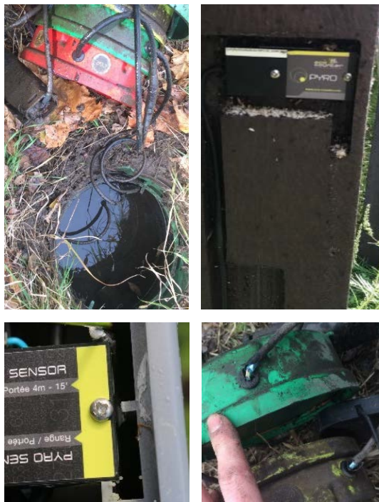
Figure 3: Examples of environmental and equipment issues. Clockwise from top left – water infiltration, ant infestation, cracked cable housings, spider web with eggs.
