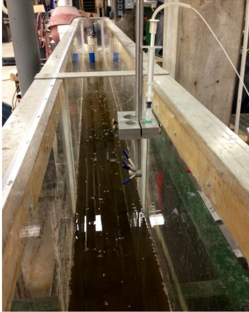
Figure 9. Flume Setup showing acoustic Doppler velocimeter (ADV) and dissolved oxygen needle for collection of oxygen microprofiles.
