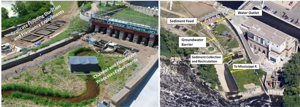
Figure 5. Layout of Outdoor StreamLab (OSL). A basin in the left photo was used to examine flooding duration and frequency in surface water storage features and the meandering channel on the right provides a field-scale channel with vegetated floodplain to investigate the impact of flooding duration and frequency in a flowing system.
