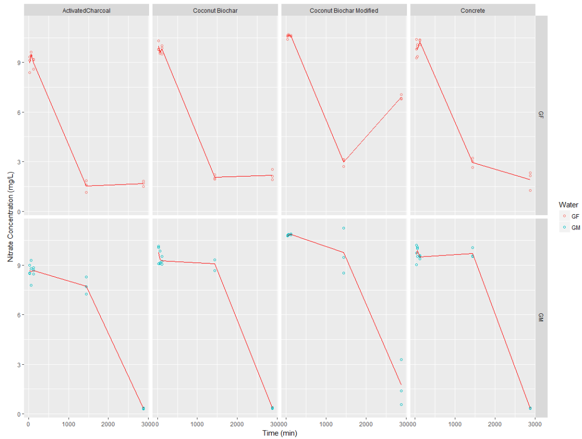
Figure 2-12. Nitrate concentration as a function of time with four materials (activated charcoal, concrete, coconut biochar, and modified coconut biochar) for the two different tile drainage waters (Grand Meadows and Granite Falls).
