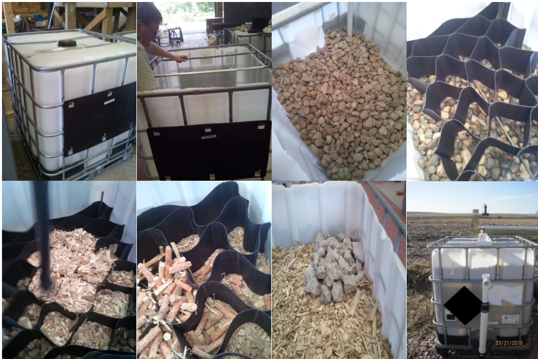
Figure 4.2. Top row from left: reinforced modular container; container with top cut off; rock layer; geotextile honeycomb material in position. Bottom row from left: filling and packing mixed woodchips; filling and packing corn cobs; crushed concrete; complete modular bioreactor deployed in the field.
